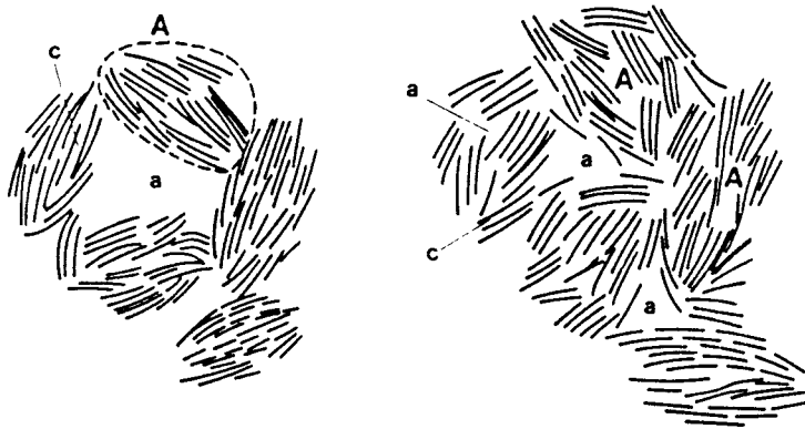
Fig 4. Schematic particle arrangement in dense bentonites: Left: Compressed granules (A) with inter-aggregate voids (a) and interlamellar space (c). Right: Homogeneous, water saturated state with expanded granules forming stacks, the voids being smaller and the interlamellar space being wider than in the initial state
