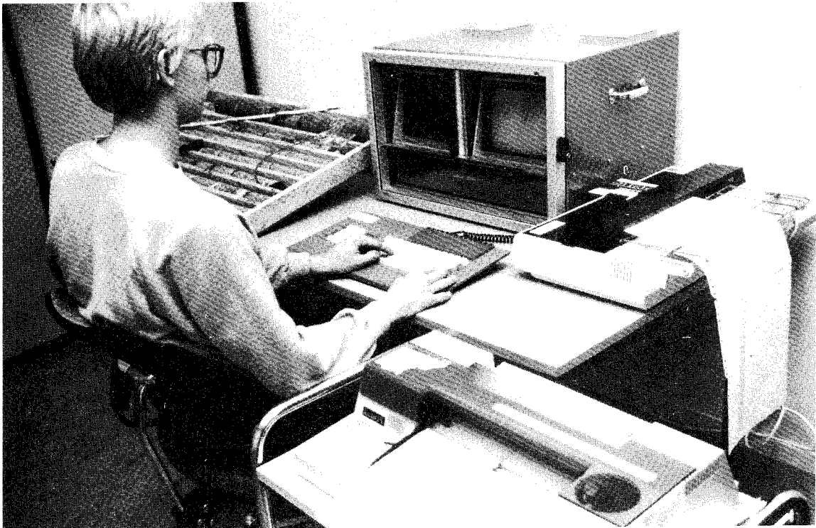
Figure 3.1 Equipment for core logging
