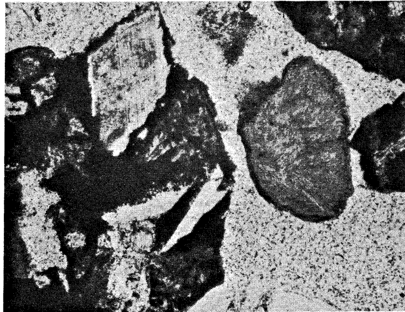
Figure 7. Single grains cemented together by Fe-oxyhydroxide. To the right a grain of basite shows a rim of clay minerals (K1 7:125.1). Photo of thin section.
