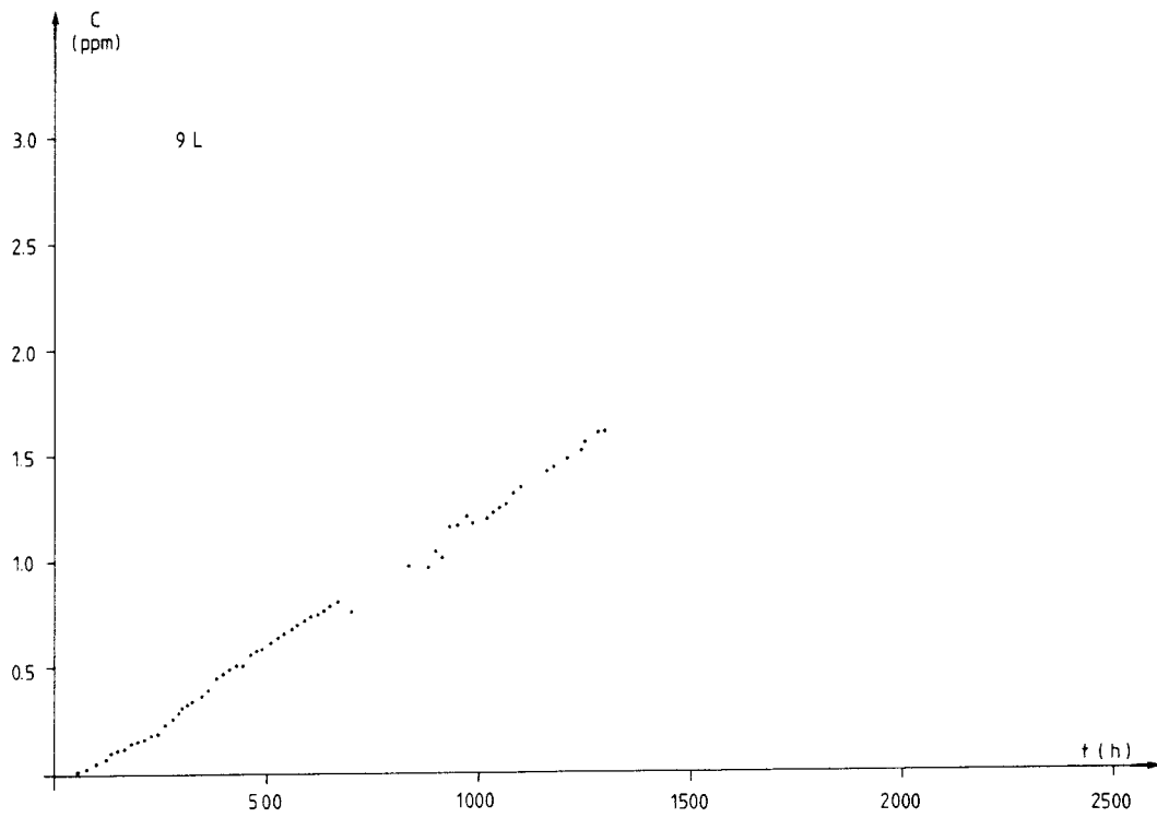
Fig 15a Breakthrough curves for Uranine in sections 3 L and 9 L.
