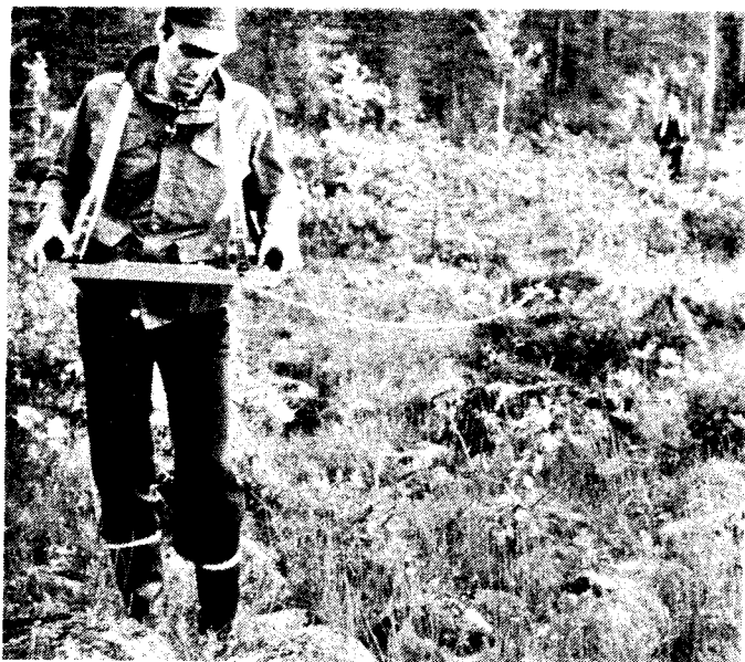
Figure 5-3. Slingram (horizontal loop EM) measurements are included in the geophysical surface measurements.
