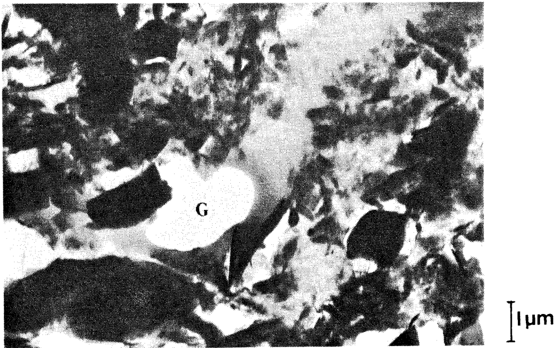
Fig.1. Electron micrograph of ultrathin section of acrylate-bedded glacial, illitic clay. G is a truncated gas pore.
