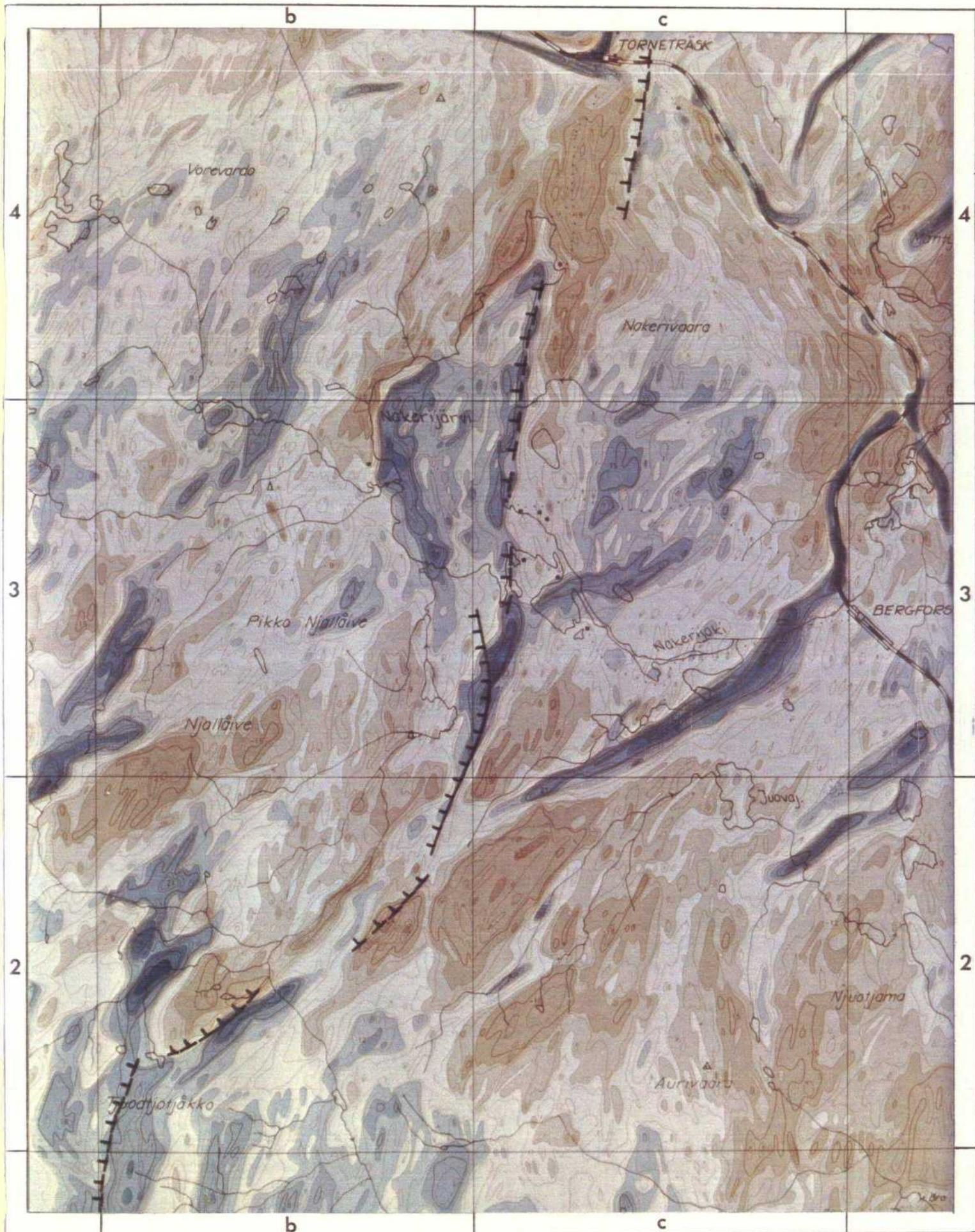
Figure 32. The appearance of the Pärvie fault on the RAMA (airborne VLF) map south of Torneträsk railway station, map area 30J SW.
