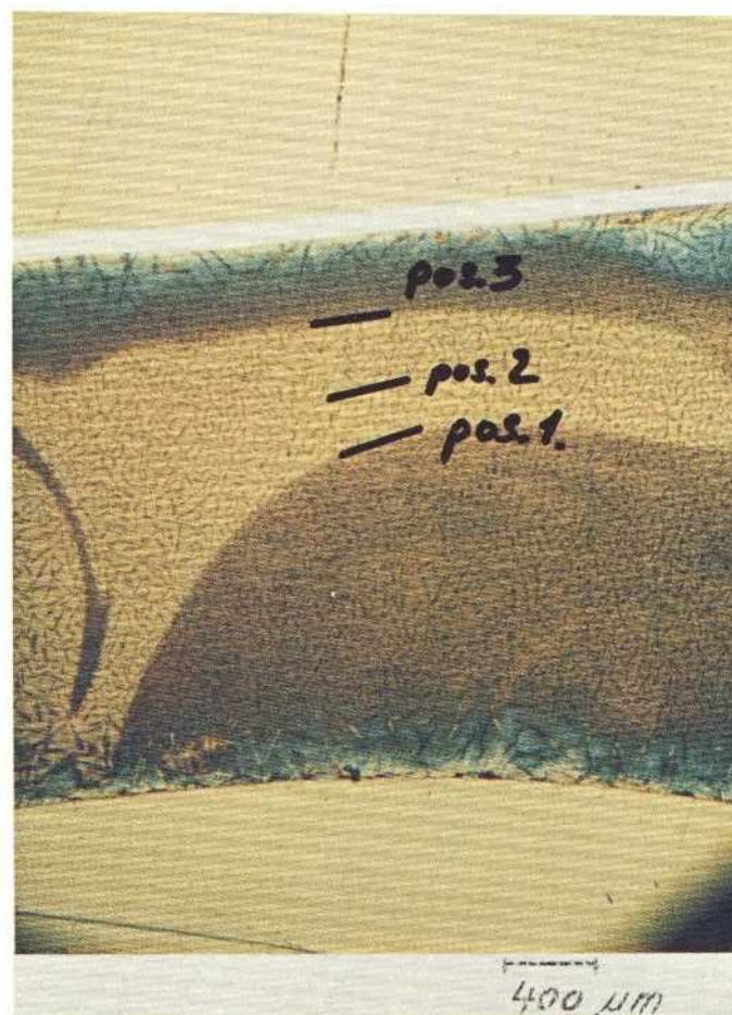
Photo micrograph of polished, HF-vapour etched sample from test series III, phase-separated in blue areas.
