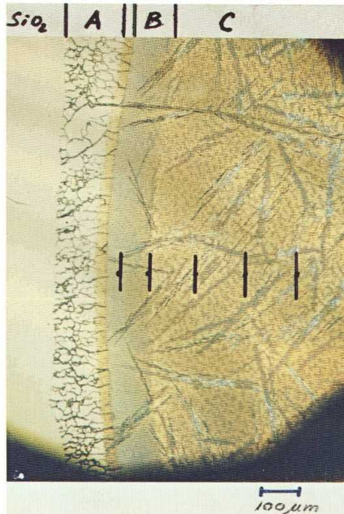
Photo micrograph of polished, HF-vapour etched sample from test series II, phase-separated in blue zone (zone B), (sample heattreated 10 min. at T_D = 1500^{\circ}\text{C} and 18 hours at T_A = 600^{\circ}\text{C} ).
