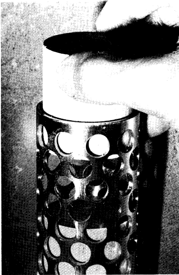
Fig.4-3. Blocks of highly compacted bentonite in a perforated metal pipe to be used for plugging of boreholes.
