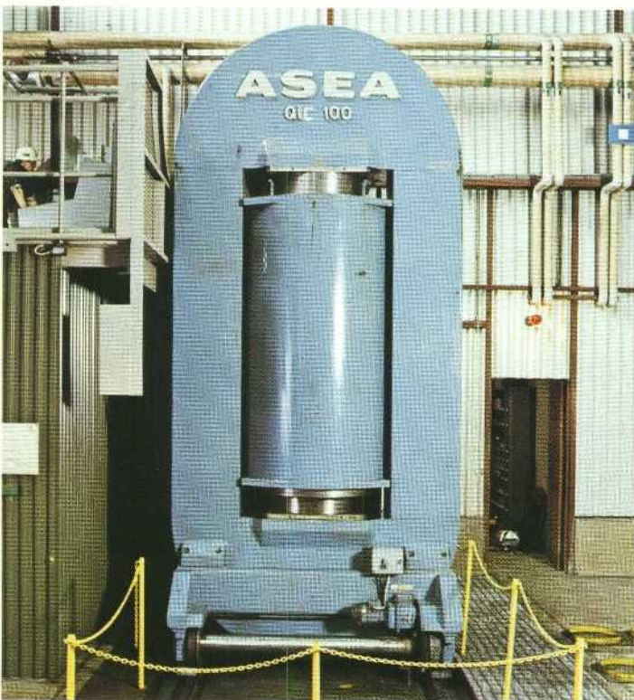
Fig. 16. For large floor-installed presses a platform can be fitted to provide a suitable work height for the operator during charging. When the press is in operation, the platform is swung up so that the frame can be moved over the vessel. (F 87889)
