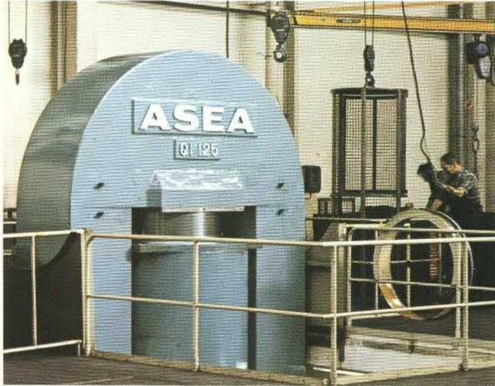
Fig. 11. When pressing, the frame is positioned over the vessel. Preparation of the next charge is usually carried out during pressurising and decompression. (F 91094)
