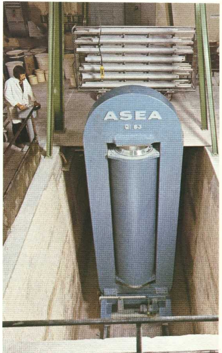
Fig. 17. QUINTUS presses can be conveniently installed at two floor levels. The top of the vessel is then positioned to give a comfortable work height at the upper floor level. The hydraulic equipment can be placed at the lower floor level alongside the press. (F 88002)
