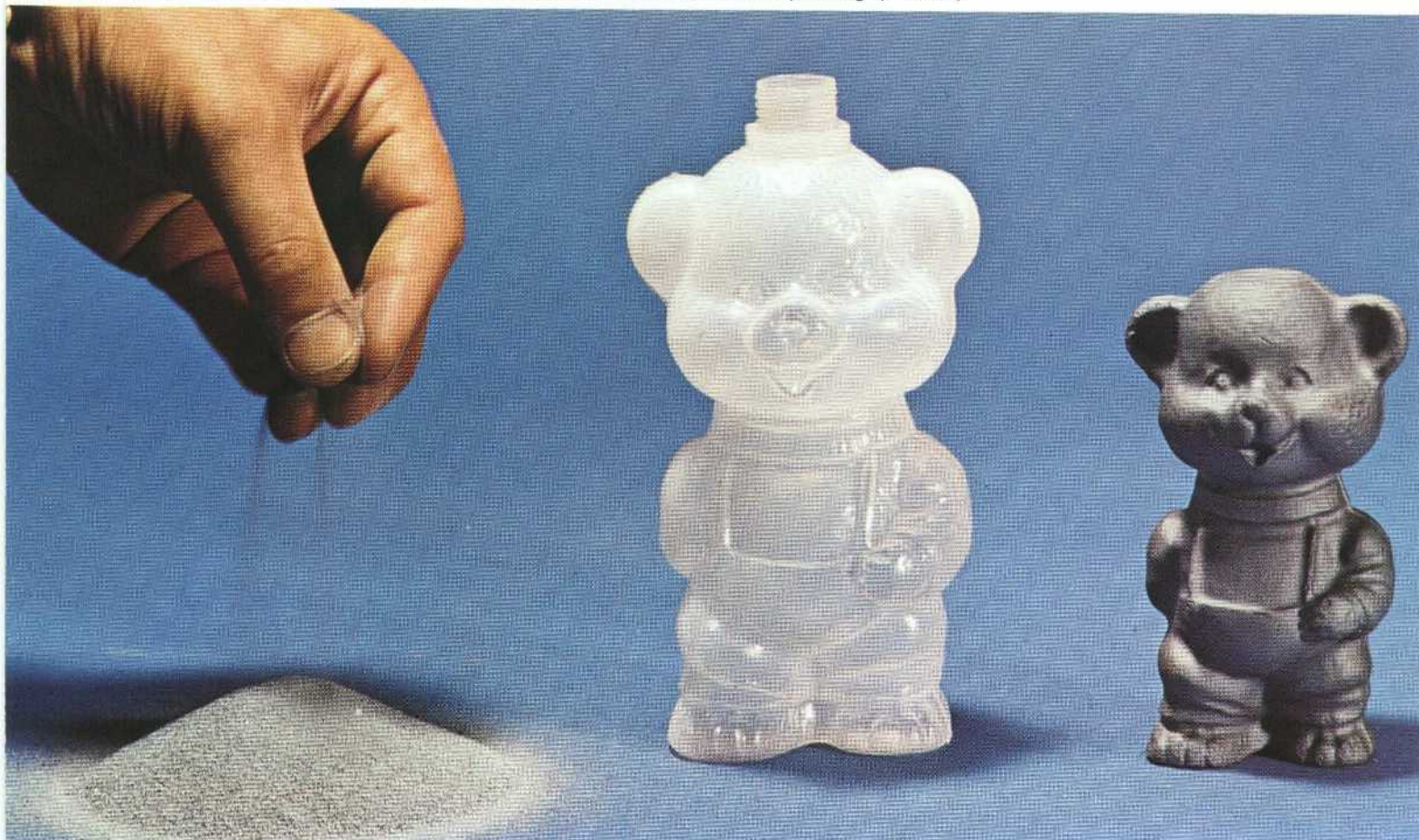
Fig. 2 Powder is pressed to complex shapes of homogenous density by isostatic pressing. (F 94151)
