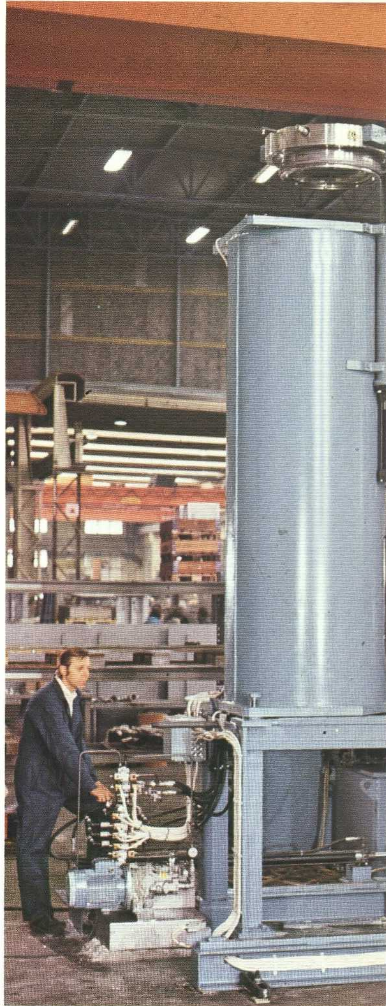
Fig. 9. QUINTUS cold isostatic presses are available as individual presses, as well as with complete auxiliary equipment.
