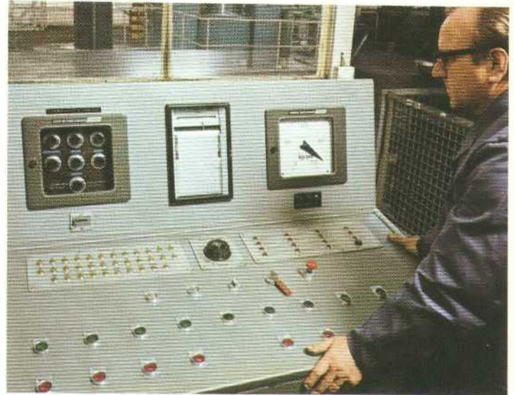
Fig. 13. Control systems are available in a number of arrangements. This operating desk has an electric precision pressure gauge, pressure recorder and controls for setting of pressure levels upon pressure rise and decompression. (F 88241)
