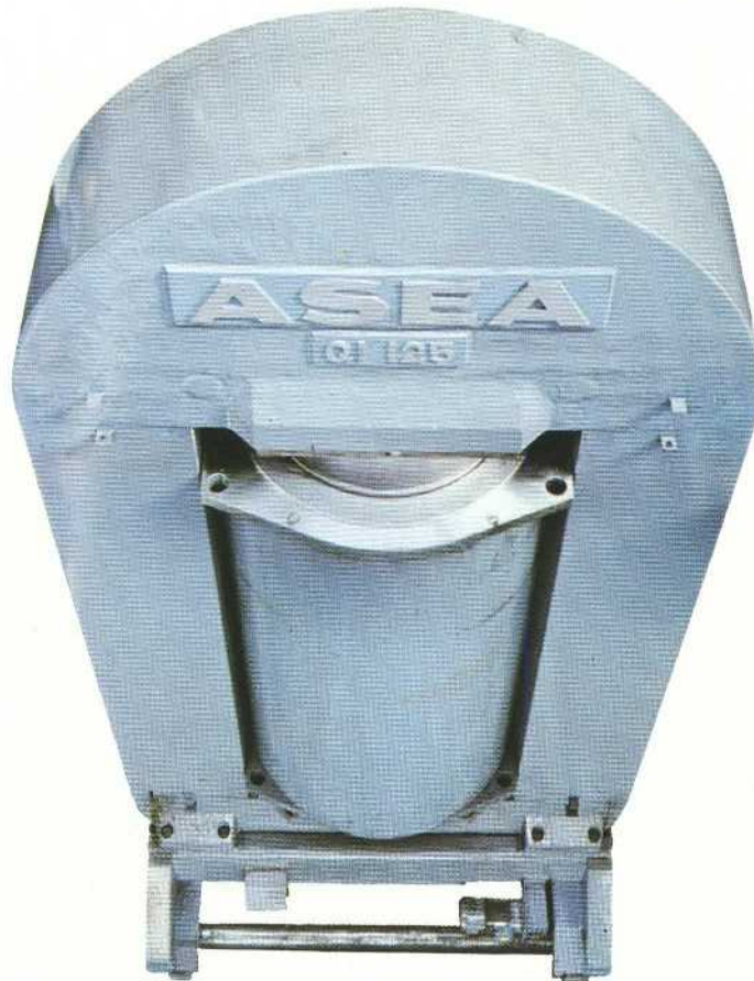
Fig. 18. QUINTUS is the trade name of ASEA's wire-wound press. Over the years, the QUINTUS concept has been extended to include the modern high pressure technique which ASEA has developed for industrial production.
