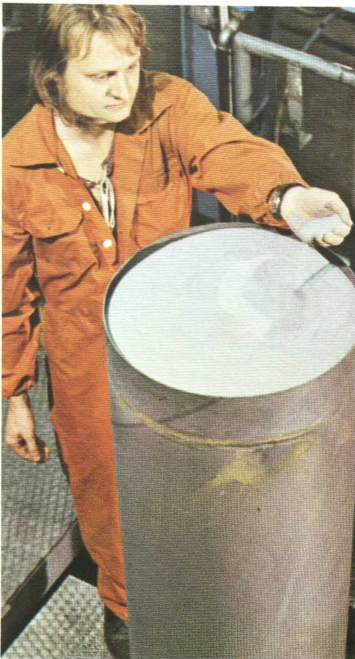
Fig. 3 Cold isostatic pressing is often used to achieve higher density in powder filling capsules prior to hot isostatic pressing. (F 94988)
