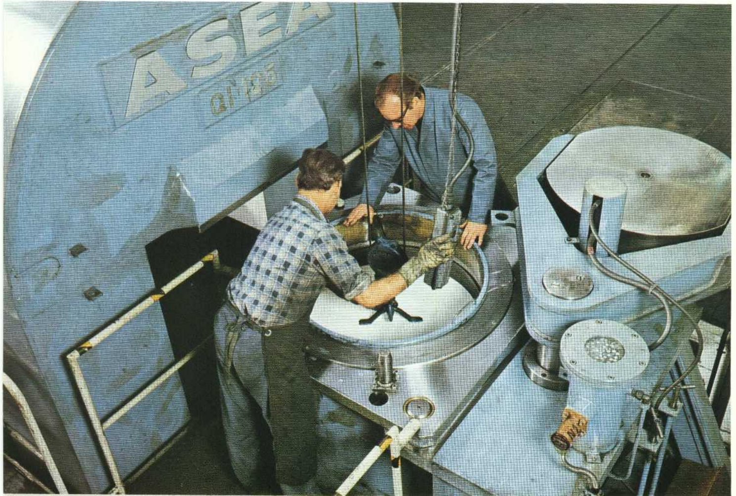
Fig. 12. When loading this QUINTUS cold isostatic press the frame is moved aside, the upper end closure is lifted and swung away, and a platform for the operator is moved forward. (F 88242)
