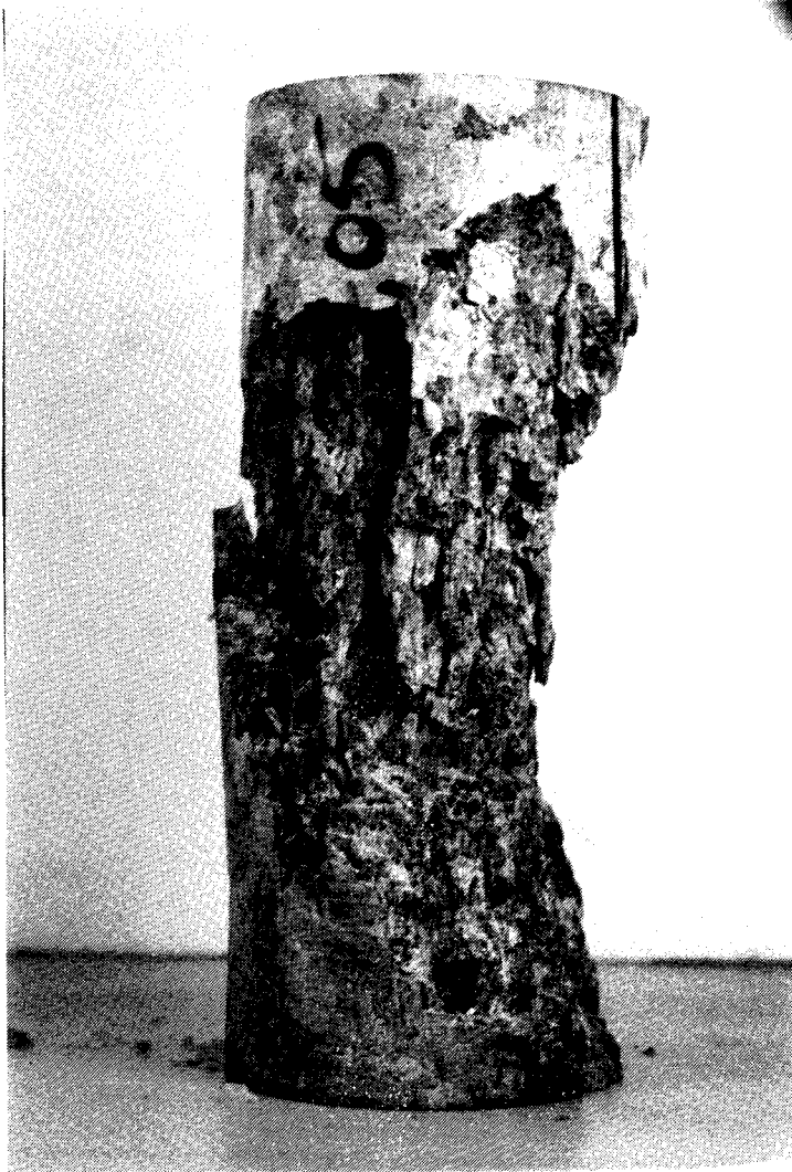
Appearance of failed specimen after uniaxial compression test: Krákemála granite.
