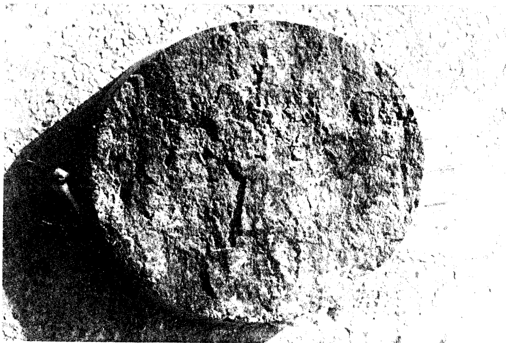
Appearance of a natural joint surface. The dark features are due to the presence of chlorite.
