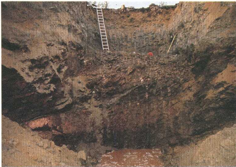
Figure 3-7. Strongly fractured and chemically weathered bedrock of the raised block at Molberget. Contact between till and bedrock in the upper part of the photograph.
