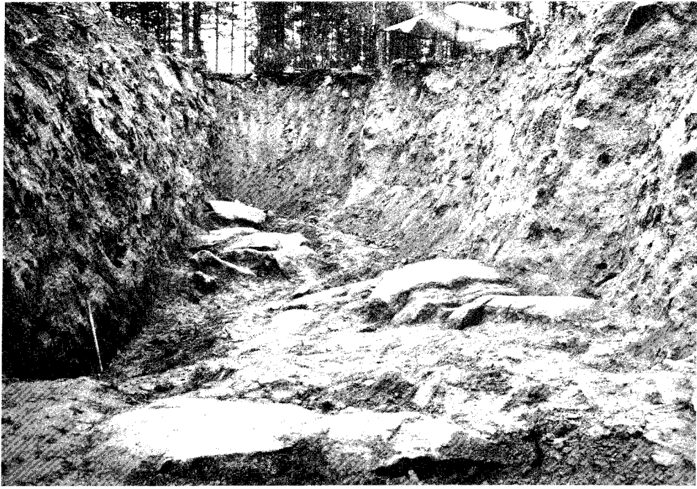
Figure 3-12. Part of the trench at Mäjärvberget showing the shattered bedrock surface on the raised block. The rock is very hard and unaffected by chemical weathering. The thickness of the till-cover is 4–5 m.
