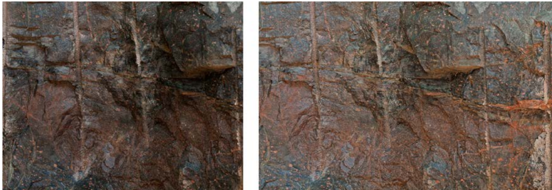
Figure 5-5. Side-by-side comparison of a close-up section of the visible light (left) and HDR (right) image. Notice the significant enhancement of detail in the shadowed areas.
