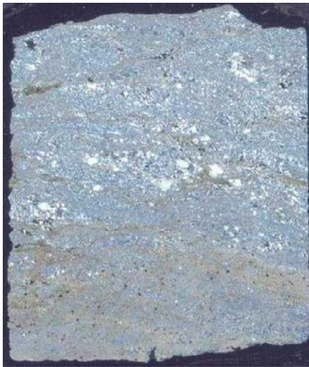
Figure 5-24. Scanned thin section. Crossed polars. Tunnel sample #7.
