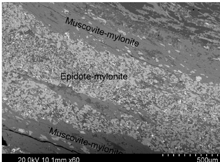
Figure 4-52. Back-scattered SEM-image showing parallel mylonite-bands either dominated by epidote or by muscovite. Uppermost part is quartz-dominated (darker mineral). Sample KI0014B01: 72.16–72.28 m.
