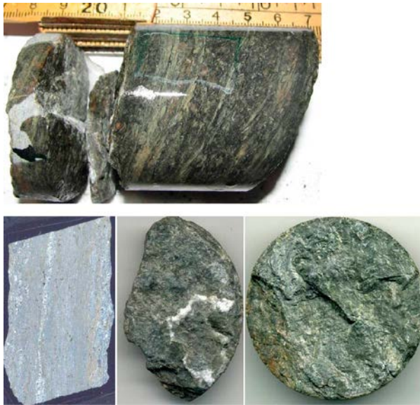
Figure 4-43. Top: Photograph showing the sample KI0010B01: 75.35–75.42 m. Bottom left: Scanned thin section, with crossed polars. Bottom right: Photographs of the fracture surface samples from KI0010B01 (1, left; 2, right).
