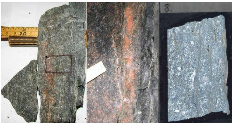
Figure 5-30. Photograph of sample (left), photograph of sample location (middle) and scanned thin section, with crossed polars (right). Tunnel sample #7.
