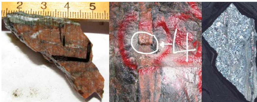
Figure 5-20. Photograph of sample (left), photograph of sample location (middle) and scanned thin section, with crossed polars (right). Tunnel sample #4.
