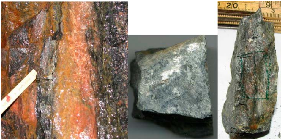
Figure 5-33. Photograph of sample location (left) photograph of fracture surface (middle), sample from the side (right). Tunnel sample #9.
