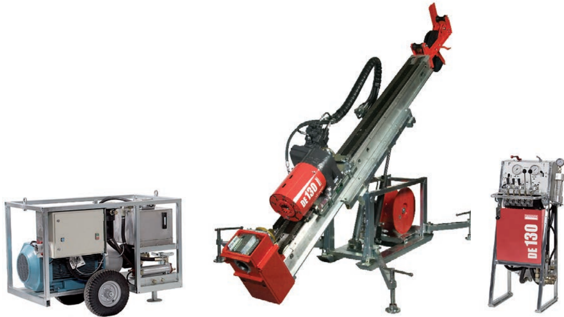
Figure 3-2. Drilling machine, Onram 1000, was used for drilling the core holes.
