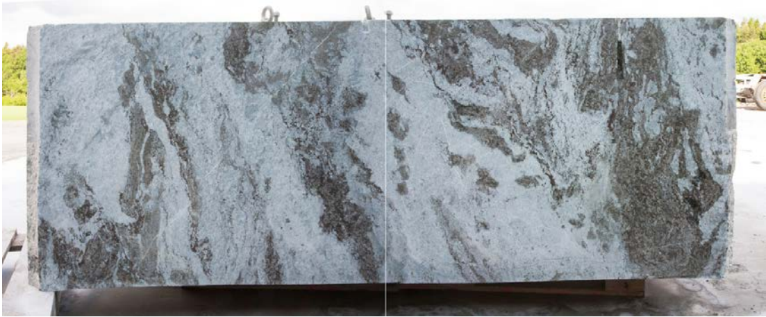
Figure 5-13. Photo of the sawn surface of the rock plug. The section is perpendicular to the tunnel direction.
