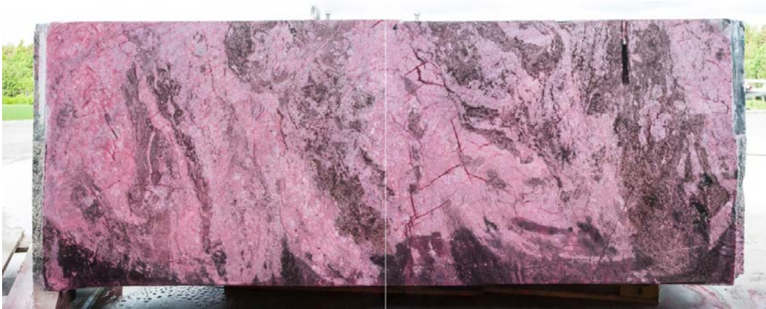
Figure 5-14. Photo of the rock plug sawn surface with penetrant.
