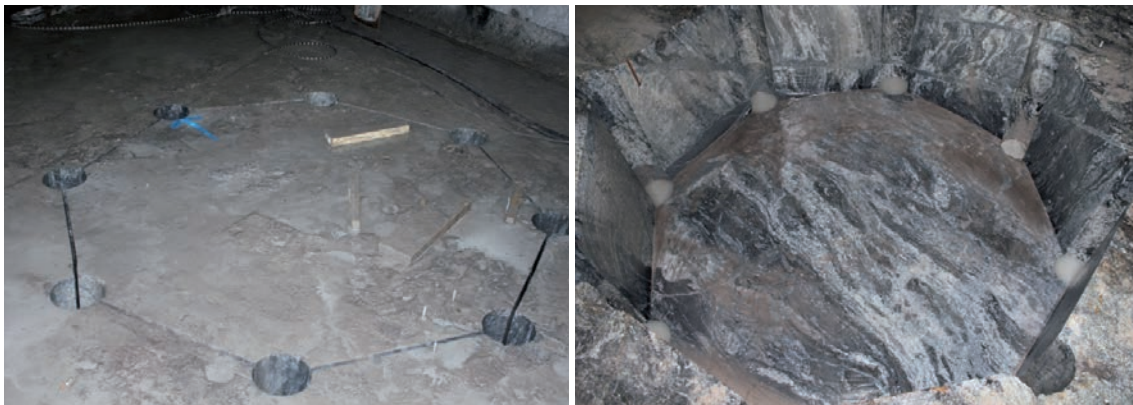
Figure 5-11. The left photo shows the drill holes and sawn sides (cf. Figure 3-9). The right photo shows appearance when the rock plug is removed.
