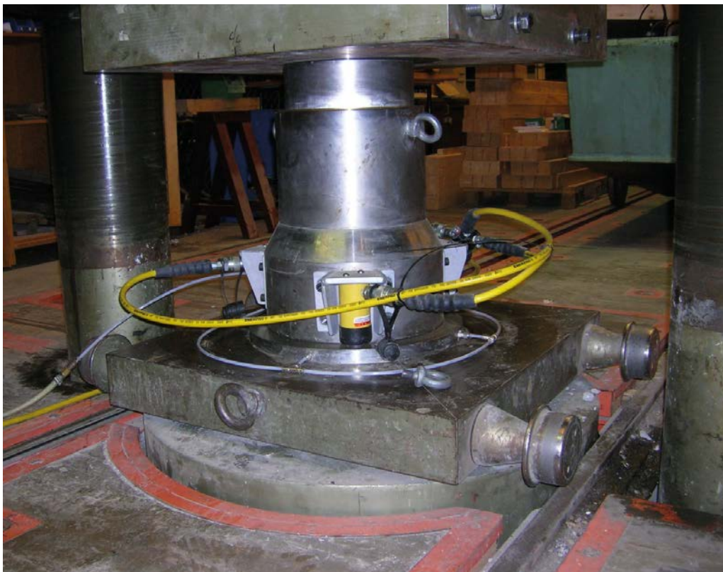
Figure 5-2. Equipment used for block compaction. The yellow tubes are for de-airing.
