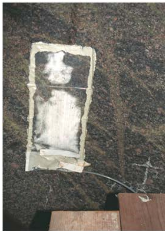
Figure 4-1. Observed fractures and water inflow into deposition hole 6 (Rhén and Forsmark 2001).
