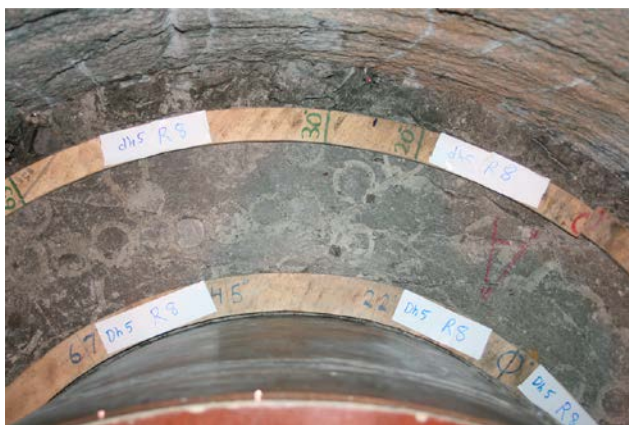
Figure 2-5. Graduated rulers placed towards the canister and the rock surface for determining the position of the samples.
