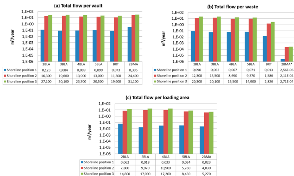
Figure 7-5. Total flow through the SFR 3 vaults, waste and loading area domains ( m^3/year ) for the Base case, for the three shoreline positions. The waste flow for the 2BMA* corresponds to the normalized flow per waste package. The vertical axis is logarithmic.
