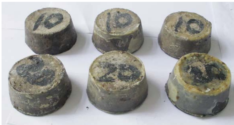
Figure 2-2. Conic specimens for the water permeability test.
