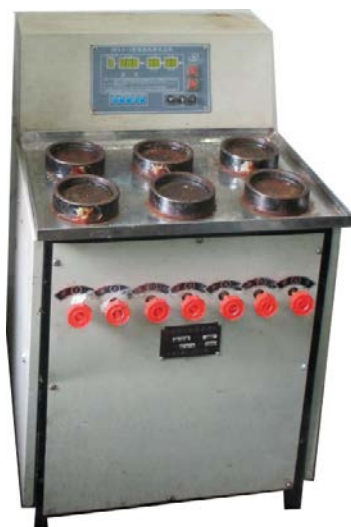
Figure C-1. Example of mortar permeameter for water permeability test.
