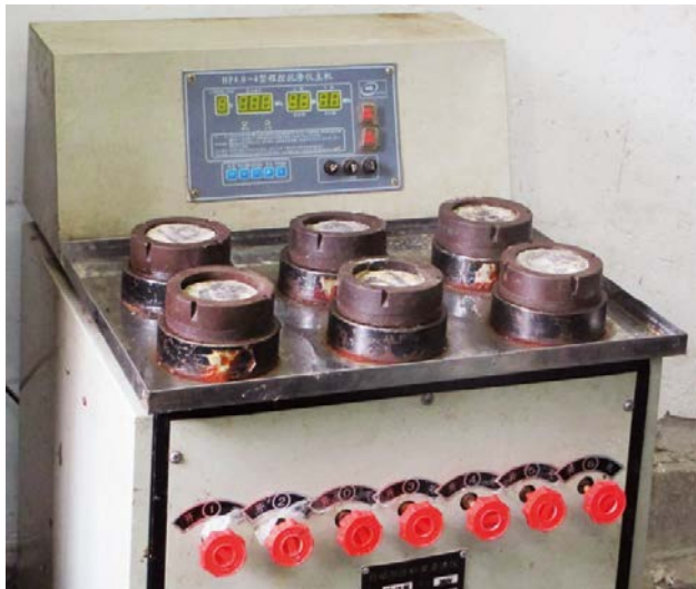
Figure 2-3. Apparatus for the water permeability test.
