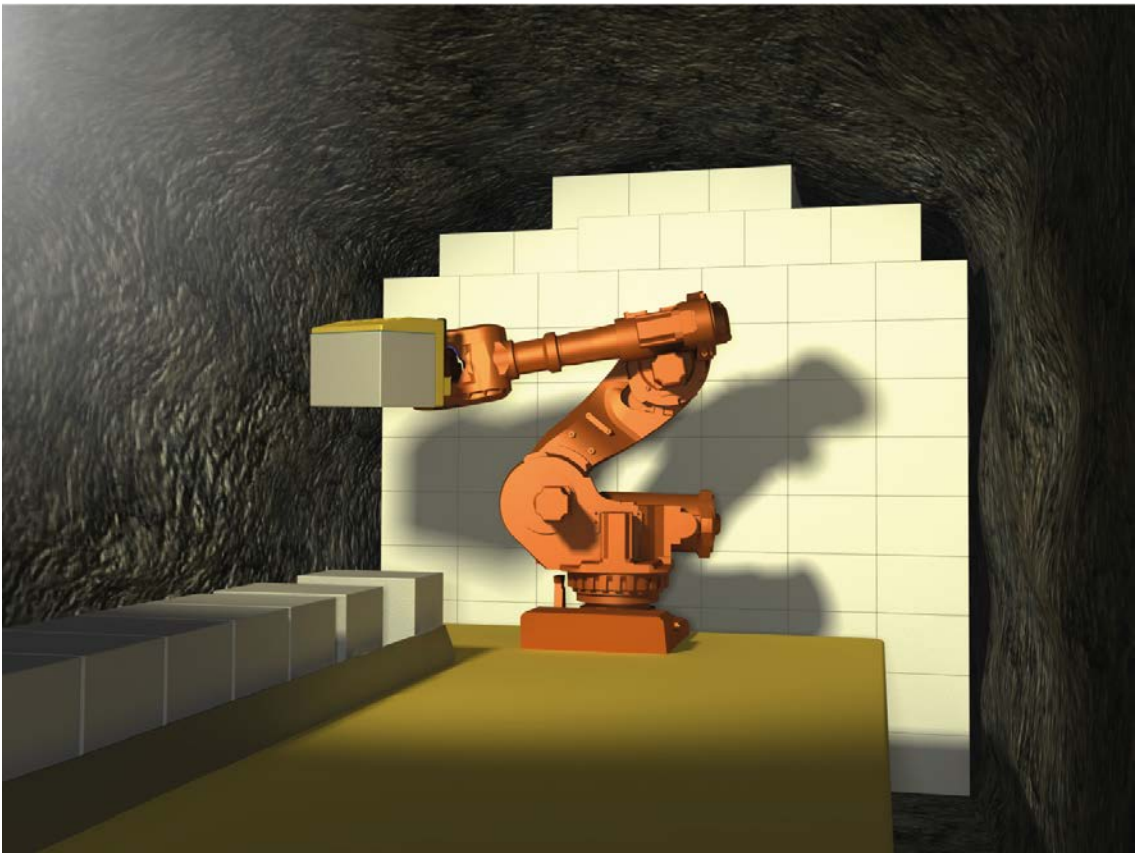
Figure 5-2. A mobile platform with a robot has been developed in order seal the deposition tunnel with backfill material and to meet the requirements.
