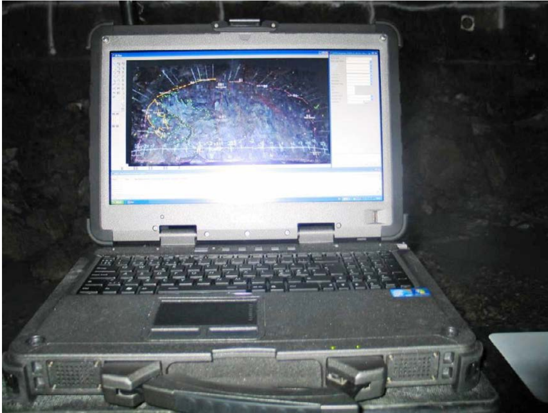
Figure 2-5. The geological features are drawn directly on the laptop screen and data are fed into the computer.
