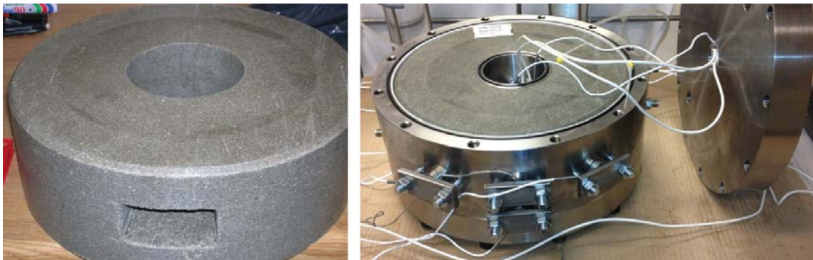
Figure 4-40. Assembly of the scale test for homogenisation modelling. The left picture shows the bentonite ring with the rectangular cavity.
