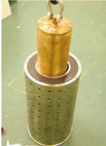
Figure 4-29. Model canister being lowered into support cage containing bentonite pellets in annulus.
