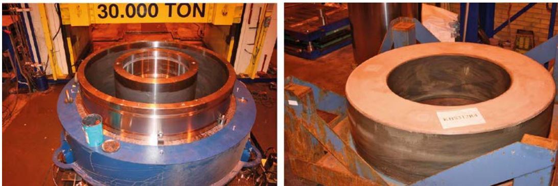
Figure 4-21. Pictures from buffer manufacturing, to the left the new KBS-3H buffer mould and to the right a compacted bentonite 'ring' which will be used in the Supercontainer around the canister. After compaction the blocks are sent to machining to the correct dimensions.
