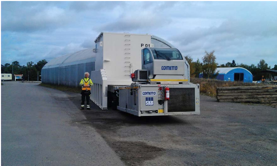
Figure 5-4. Ramp Vehicle carrying the modified ATB.
