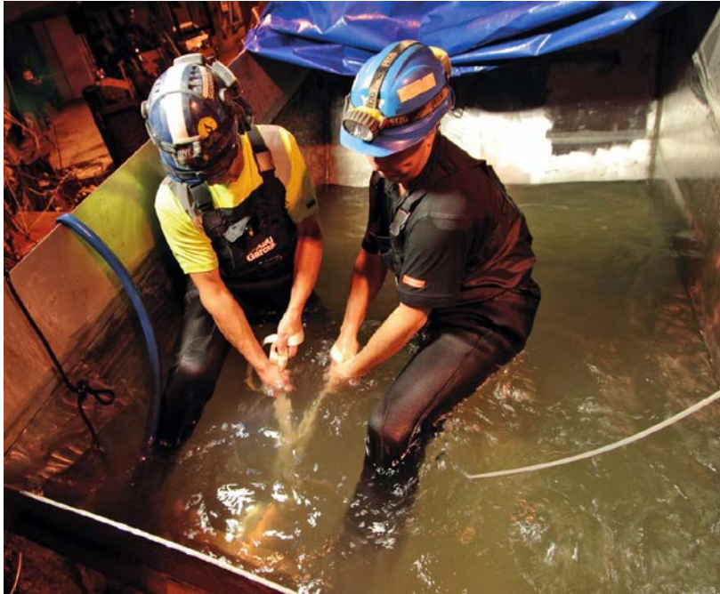
Figure 4-31. Stefan Grandin Svårdh and Jonas Hallberg pulling out the steel cage from the KA3386A04 bore hole.
