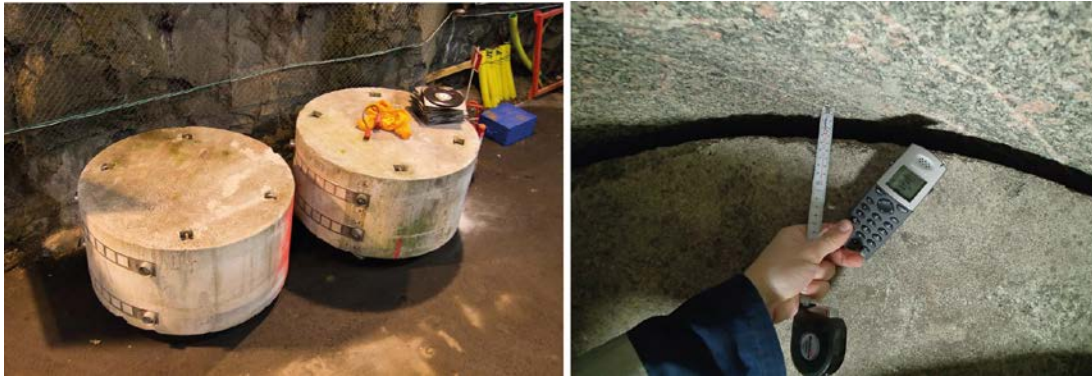
Figure 4-20. To the left dummy distance blocks with the newly designed feet mounted and to the right the same blocks after deposition tests inside the drift, also illustrating the tight fit between the drift wall and the components.
