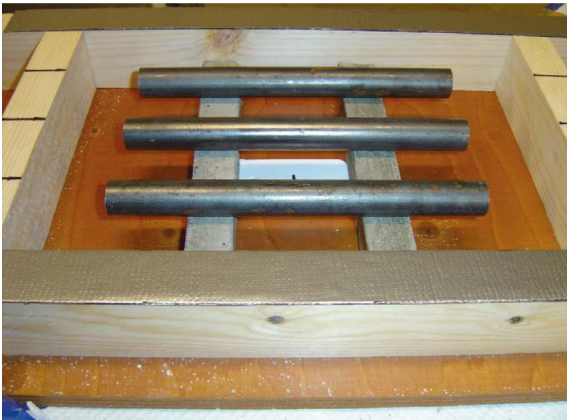
Figure 4-37. Mould and steel bars on supports before casting.
