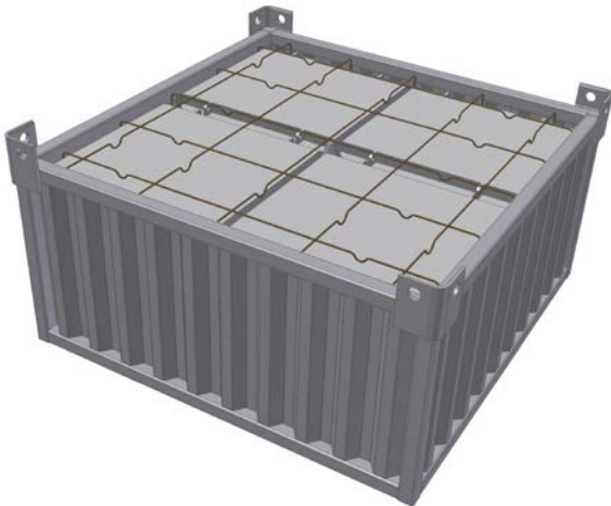
Figure 5-6. Waste container for waste currently stored in moulds. The lateral dimensions are the same as for the containers shown in Figures 5-2, 5-3 and 5-5. The height of the container is 1.30 metres. The moulds are stabilized in the container with grout. This container also has no lid, since the grout is intended to fill the full volume of the container. Reinforcement bars to improve the mechanical properties of the grout are shown in the figure.
