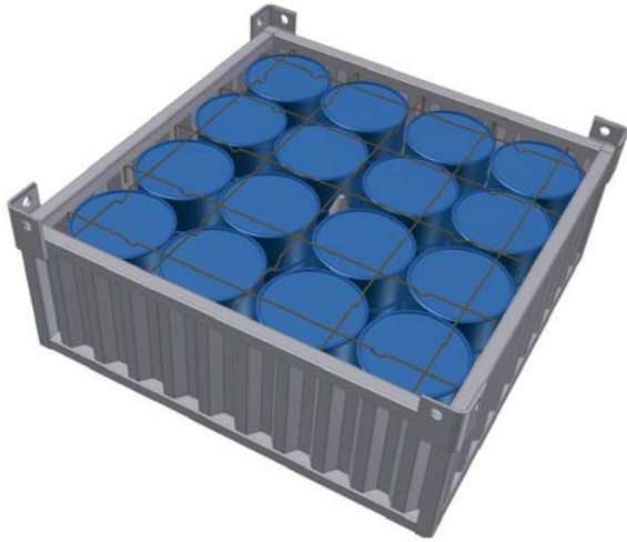
Figure 5-5. Waste container for waste currently stored in 200-litre drums. Its lateral dimensions are 2.69 metres \times 2.69 metres, which is the same as for the containers shown in Figures 5-2, 5-3 and 5-6. The height of the container is 0.96 metre. The drums are stabilized in the container using grout. The container has no lid, since the grout is intended to fill the full volume of the container. Reinforcement bars to improve the mechanical properties of the grout are shown in the figure.
