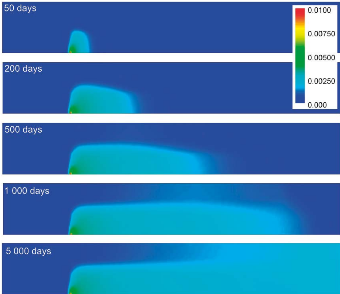
Figure 4-9. Tracer concentrations (mol/L) during transient stage of migration in the till calculated for the 3-layer till model. The initial tracer concentration in the deep groundwater was arbitrarily set to 0.1 mol/L.
