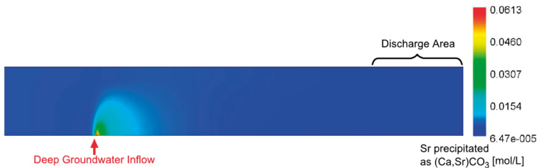
Figure 4-31. Base Case Sr precipitation as (Ca,Sr)CO_3 at the end of the simulation (2,700 years after the onset of injection).
