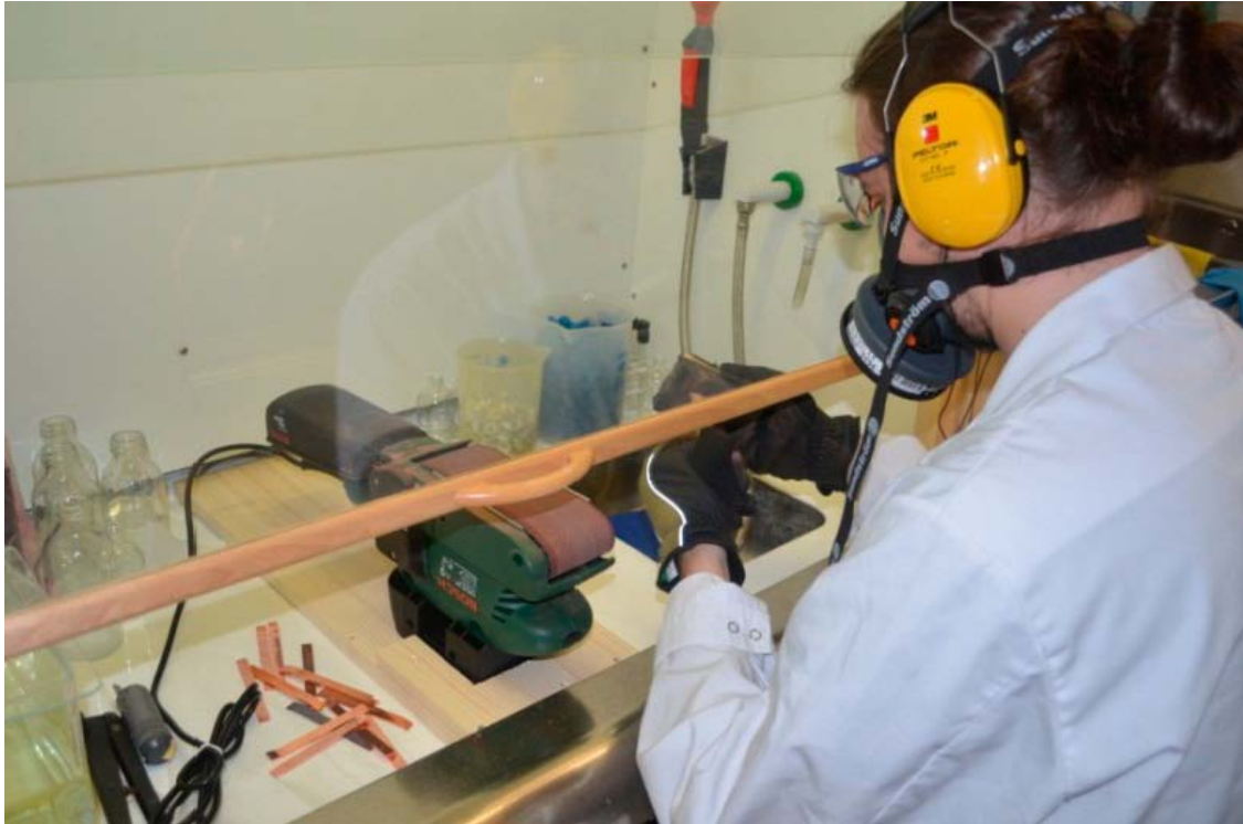
Figure 3-1. Grinding surfaces of copper rod, starting with the grinder and then by hand.
