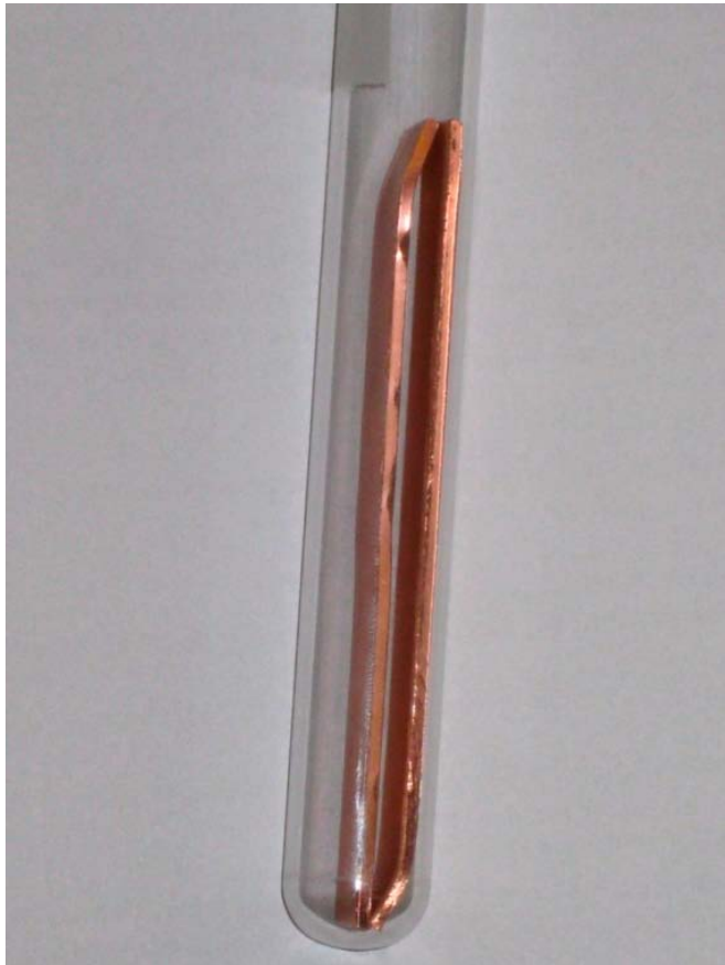
Figure A1-2. Copper rod design with 15 degree angle at one side to avoid contact between the rod surfaces.
