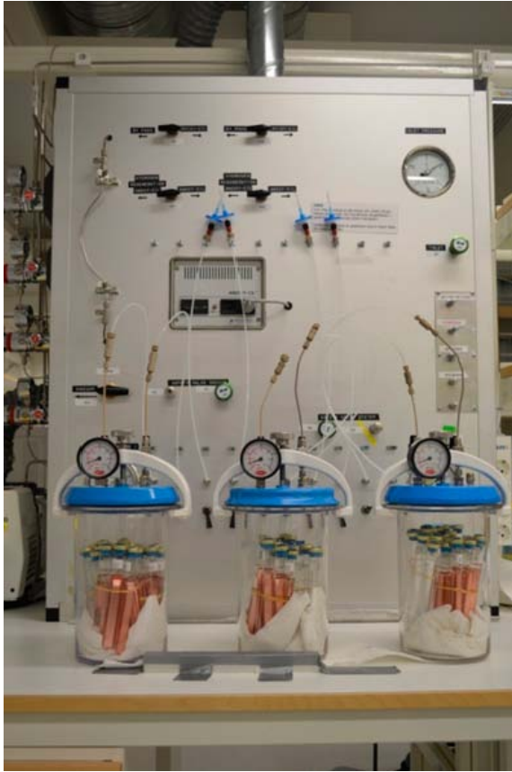
Figure 3-9. The anaerobic jars are evacuated and filled with N 2 at the Gas bench.
