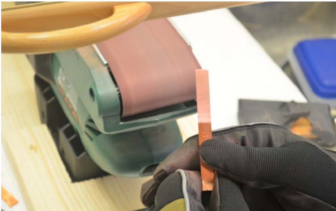
Figure 3-2. The upper part of the copper rod has shiny metallic surface of pure copper.
