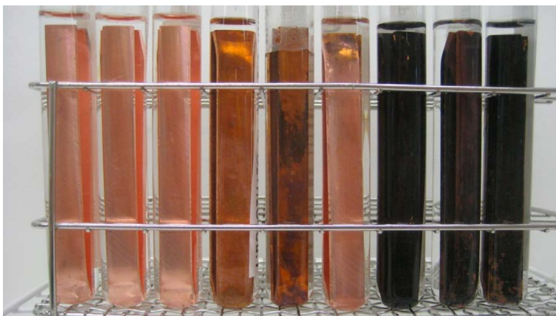
Figure A1-1. Copper rods from pilot test one exposed to varying amount of O_2 . From left to right, 0 nmol O_2 (vials 1–3), 420 nmol O_2 (vials 4–6) and 4,600 nmol O_2 (vials 7–9).
