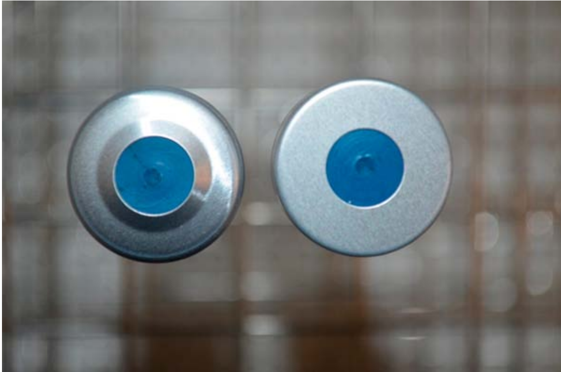
Figure 3-5. Aluminum ring to the left is correctly clamped to make sure the vial is tightly sealed.
