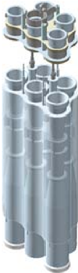
Figure 3-2. Illustration of Steam Separators after a cut.
