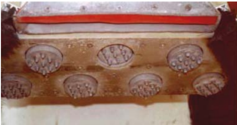
Figure A1-15. View of underside of PENTEK Moose cutting head.
