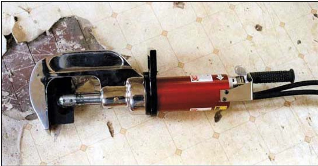
Figure A1-12. Mega-Tech Services Inc. Blade plunging cutter.
