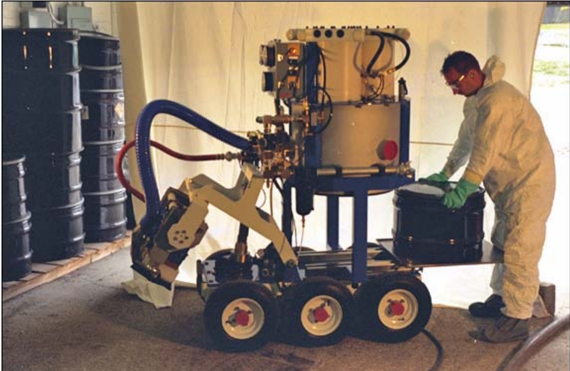
Figure A1-14. PENTEK Moose® Remotely Operated Floor Scabbler.
