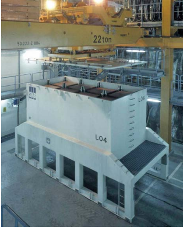
Figure 3-14. Swedish shielded transport container (Photo: Bengt O Nordin, SKB).
