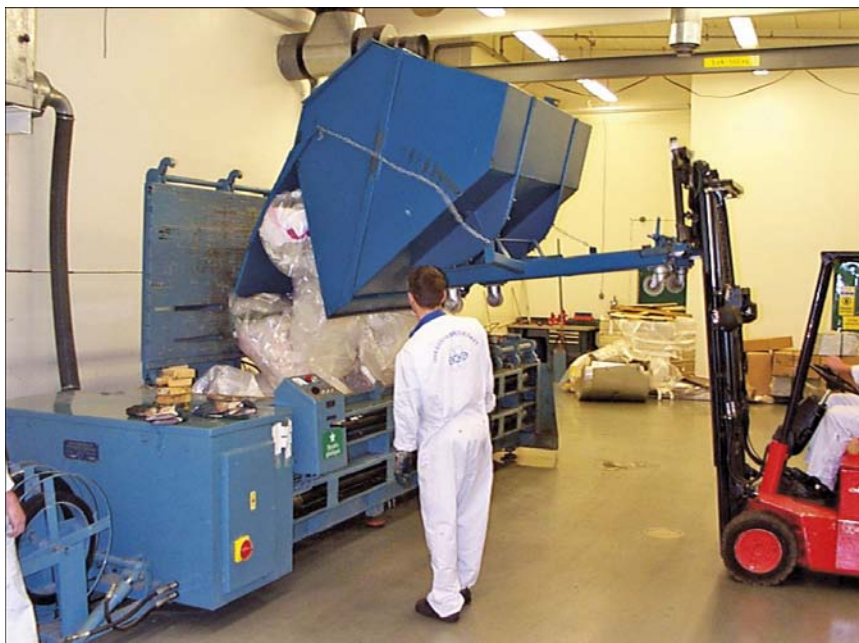
Figure A1-23. Compaction of soft LLW into square bales at Oskarshamn.
