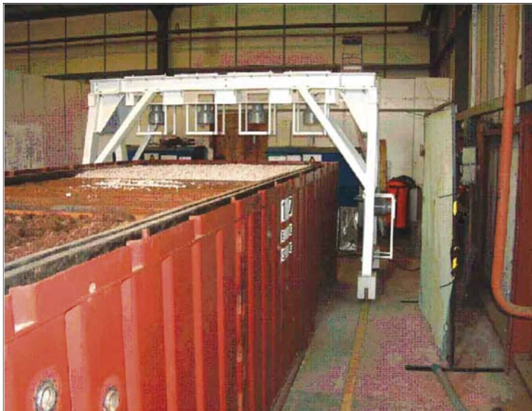
Figure A1-27. ISO Container Monitor for Bulk LLW.
