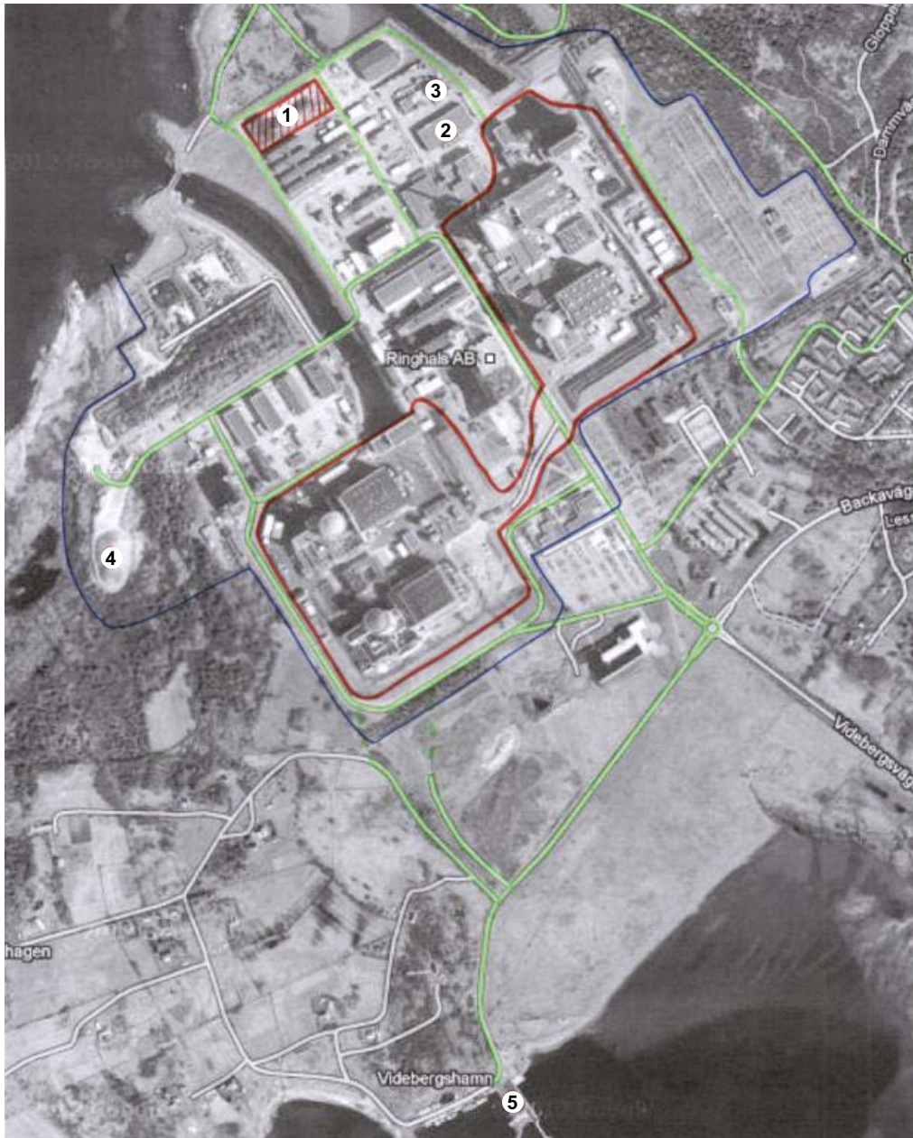
Figure B-1. Layout of the Ringhals site. The blue line delineates the industrial area and the red line the operating area. The green line represents the transport route options. Area no. 1 shows the required storage area for the waste from decommissioning of Ringhals 1–4. No. 2 shows storehouse “Kokillförrådet”, no 3. the mausoleum, no. 4 the surface repository and no.5 shows the Ringhals port, Videbergshamn.
