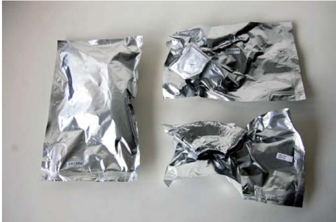
Figure 3-8. Evacuated tri-laminate bags with the two sensor pairs (and another bentonite piece).
