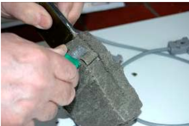
Figure 3-11. Removing bentonite by knife to make one side of the resin plate visible (cut 1).
