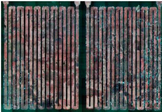
Figure 4-5. Appearance of sensor ER2 (top) after removal of the adjacent bentonite piece and (bottom) after the first ultrasonic cleaning in 10% sulphuric acid solution.
