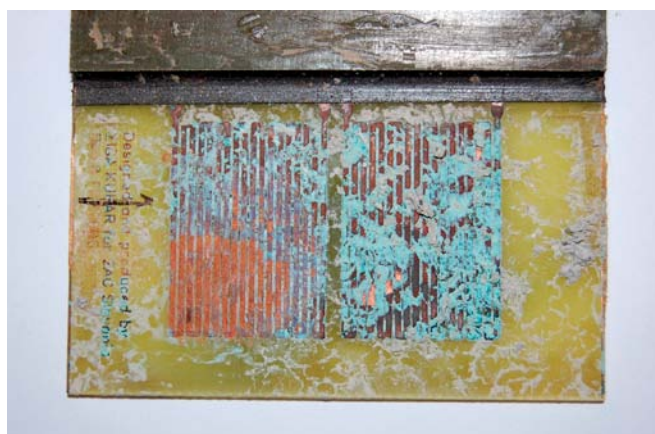
Figure 4-2. The appearance of sensor ER1 after removal of corrosion products from part of the left sensor element (the brownish area).
