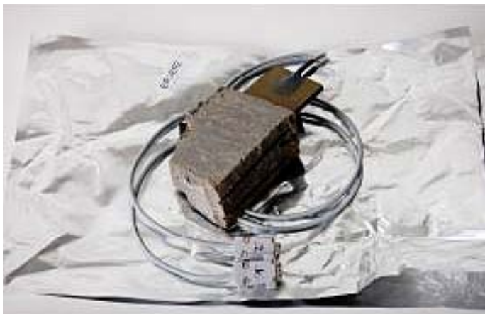
Figure 3-9. Photo of sensor pair ER1/ER2 on top of its tri-laminate bag.
