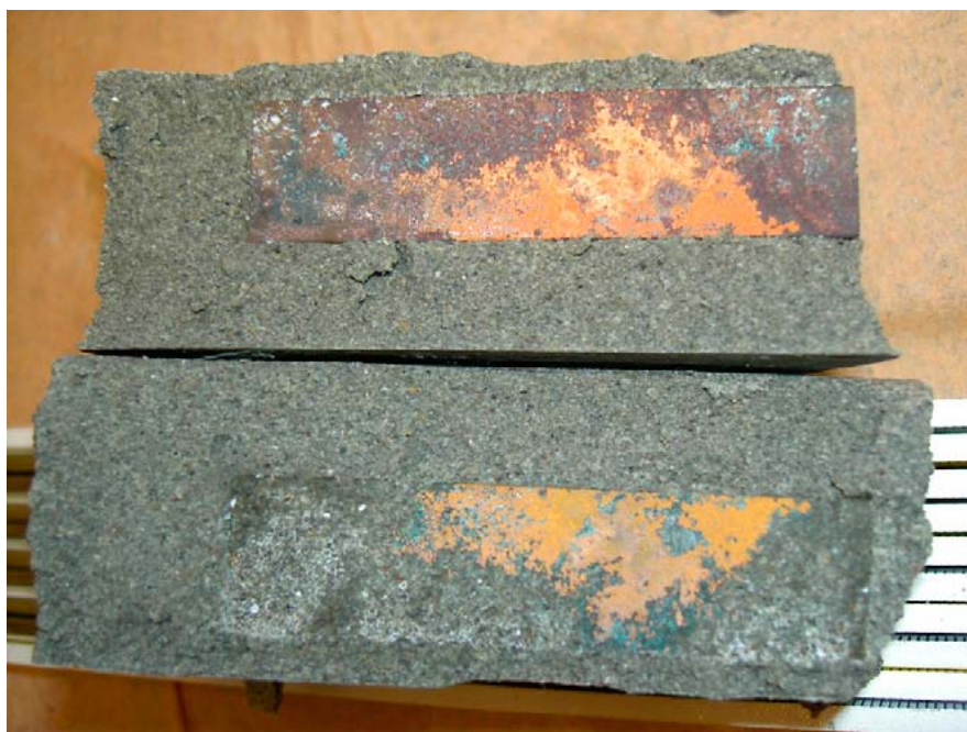
Figure 2-1. Appearance of a copper coupon after exposure in the Äspö HRL.
