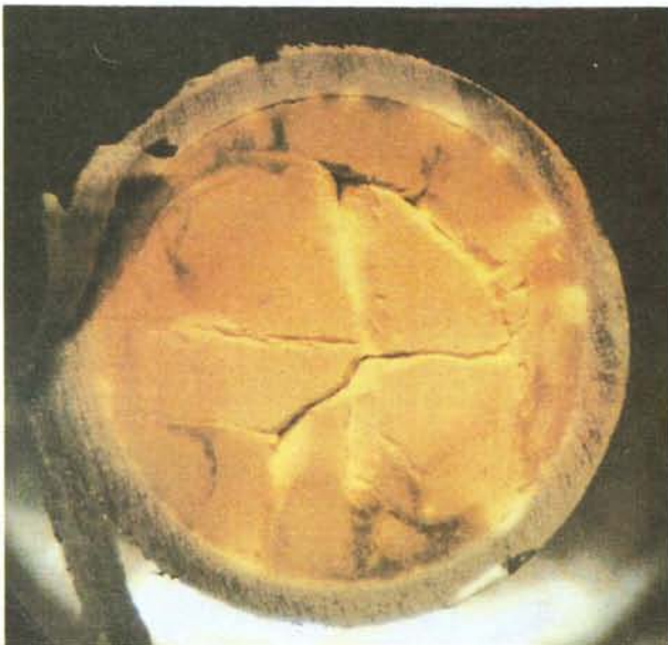
Figure 11-1. Fuel/Clad segment of PWR fuel specimen after 436 days in deionized water and 5 months of air storage
