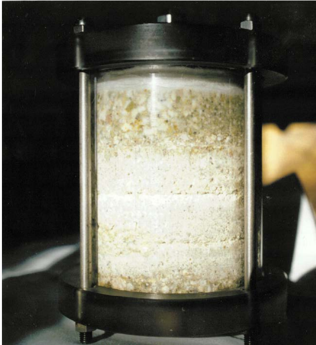
Figure A-75. Perspex cell used in joint sealing tests.
