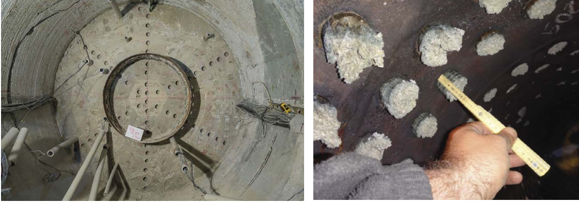
Figure 2-17. Left: Example of sampling section. Right: Bentonite bulges inside the liner (García-Siñeriz et al. 2016).
