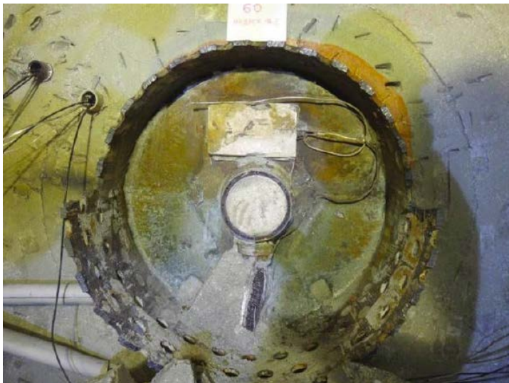
Figure B-6. View of the heater #2 before its extraction. Part of the steel lining is also visible (García-Siñeriz et al. 2016).
