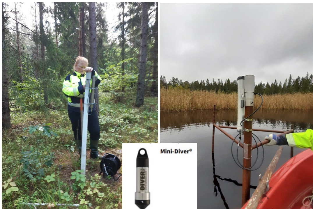
Figure 2-1 Two types of locations of groundwater monitoring wells; SFM000181 installed in forest (left), and SFM000184 with the well screen installed in regolith the bottom of a pond (right). A Mini-Diver pressure transducer (insert) was used to record changes in the pressure head over time.
