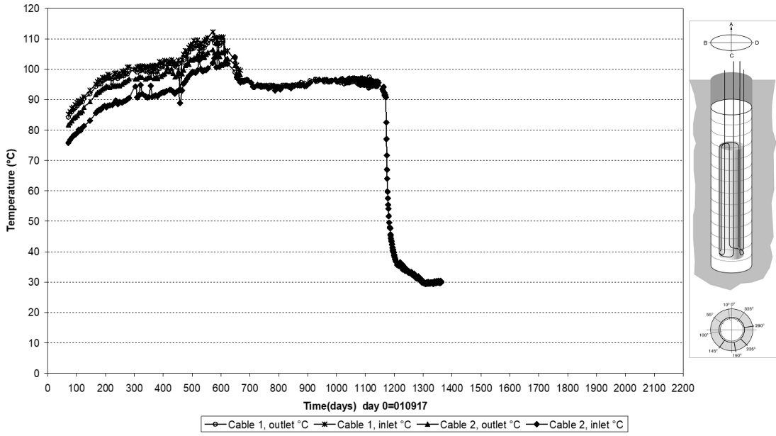
Prototype\ Hole 2 \Canister (010917-070601) Max. temperature on the canister surface - Optical fiber cables
