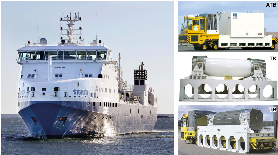
Figure 2-9. M/S Sigrid and transport casks for short-lived radioactive waste (ATB), for core components (TK) and spent fuel assemblies (TB).
