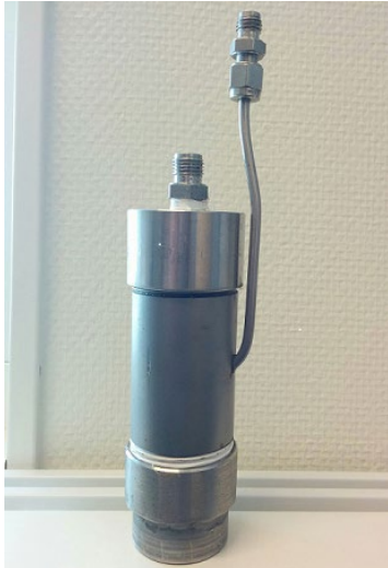
Figure 2-4. The docking unit, which is used together with the pump (GEOPUMP UV-45). Instead of using the mini-packer to isolate the lower part of the standpipe with the pump, the unit is tightly fitted to the tube in the bottom of the standpipe. The photo shows the docking unit used in normally equipped boreholes. The one used in KFM08D is modified to match with the special equipment in PEEK, but is very similar to the one in the photo.
