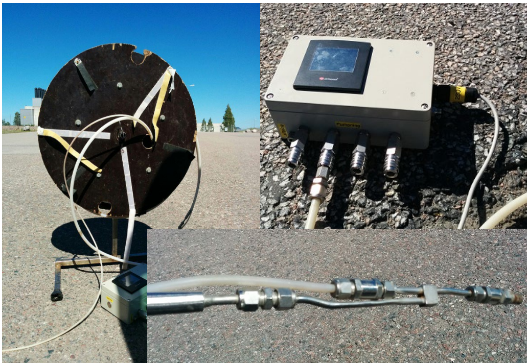
Figure 2-5. The equipment used for gas-lift pumping. On the left, the tubing lowered down the standpipe (the narrower tube for sample water and the wider for gas) on a bobbin to simplify the lowering. To the upper right the control unit for the pumping/gas supply and lower right the end of the gas-lift pump.
