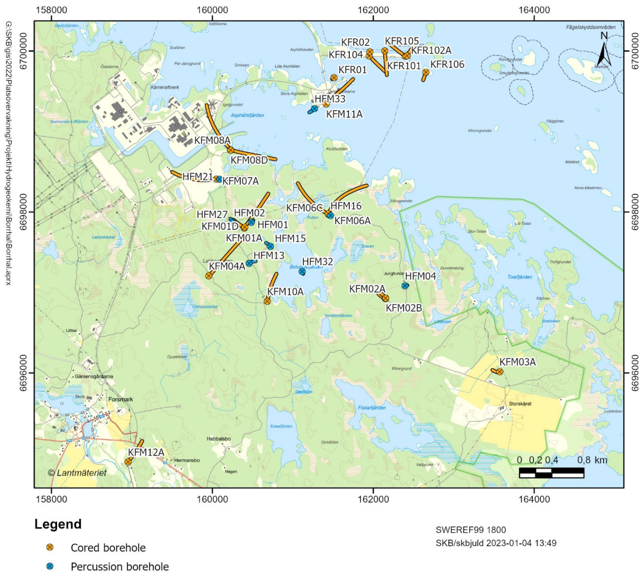
Figure 1-1. General overview of the Forsmark area and the boreholes included in the hydrochemical monitoring program for deep groundwater. The cored boreholes and the percussion boreholes within the monitoring program are marked with orange and blue filled circles, respectively. Cored boreholes drilled from the SFR-tunnel are KFR01, KFR02 and KFR105.
