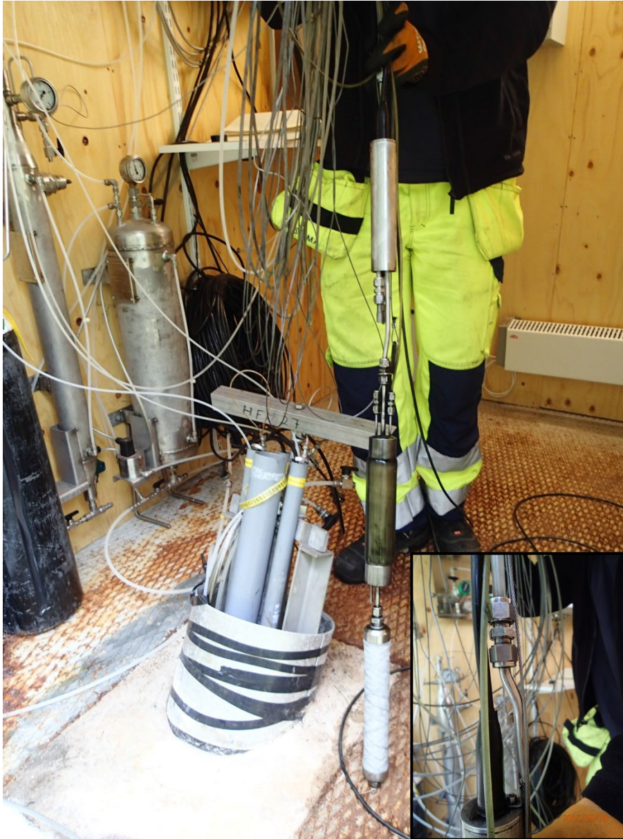
Figure 2-3. The pumping equipment (GEOPUMP UV-45) used for pumping in wide standpipes. The equipment consists of a filter and a pump connected to the mini-packer. The small diameter plastic hose is used for expanding the packer and the plastic hose connected to the pump is the pumping hose (enclosed picture right lower corner).
