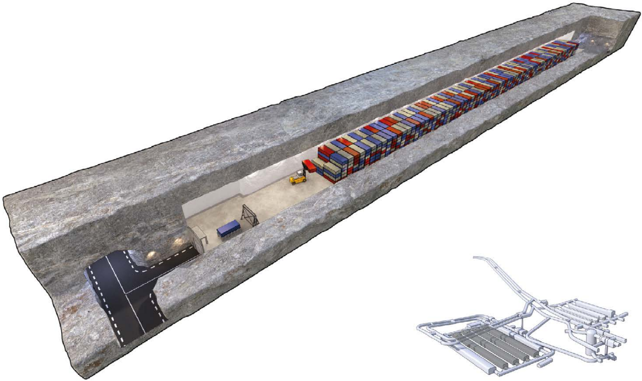
Figure 4-20. Vaults for low-level waste, 2-5BLA, in SFR3 during the operational period. The lower detail shows SFR with the position of the four waste vaults in darker grey.
