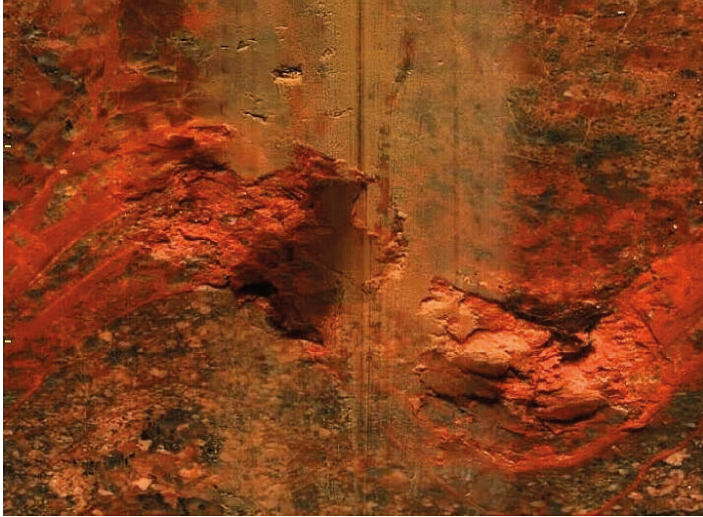
Figure 5-12. The brecciated fault rock at 106.642–106.798 m in KFR119.
