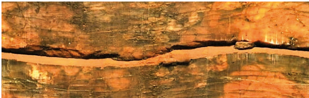
Figure 5-15. The widest fracture in KFR120 at 15.31 m, with an aperture of 6 mm.
