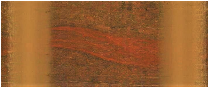
Figure 5-16. A brecciated fault rock at 61.346–61.428 m in KFR120.
