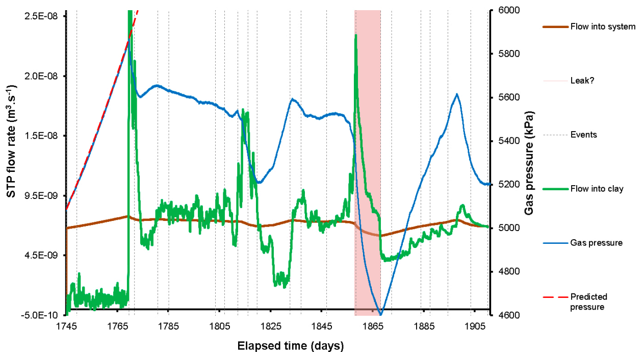
Figure 8-27. Flow of gas into the system and the clay during the fourth ramp of Gas Injection Test 2.
