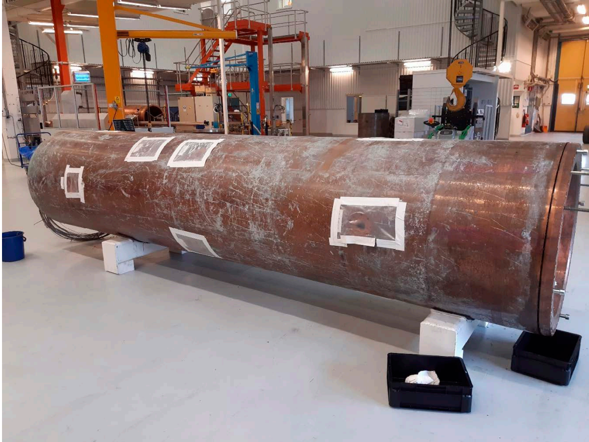
Figure 15-29. The Lasgit canister seen within the Äspö laboratory. White taped area cover the removed canister filter housings or stress sensor housings.
