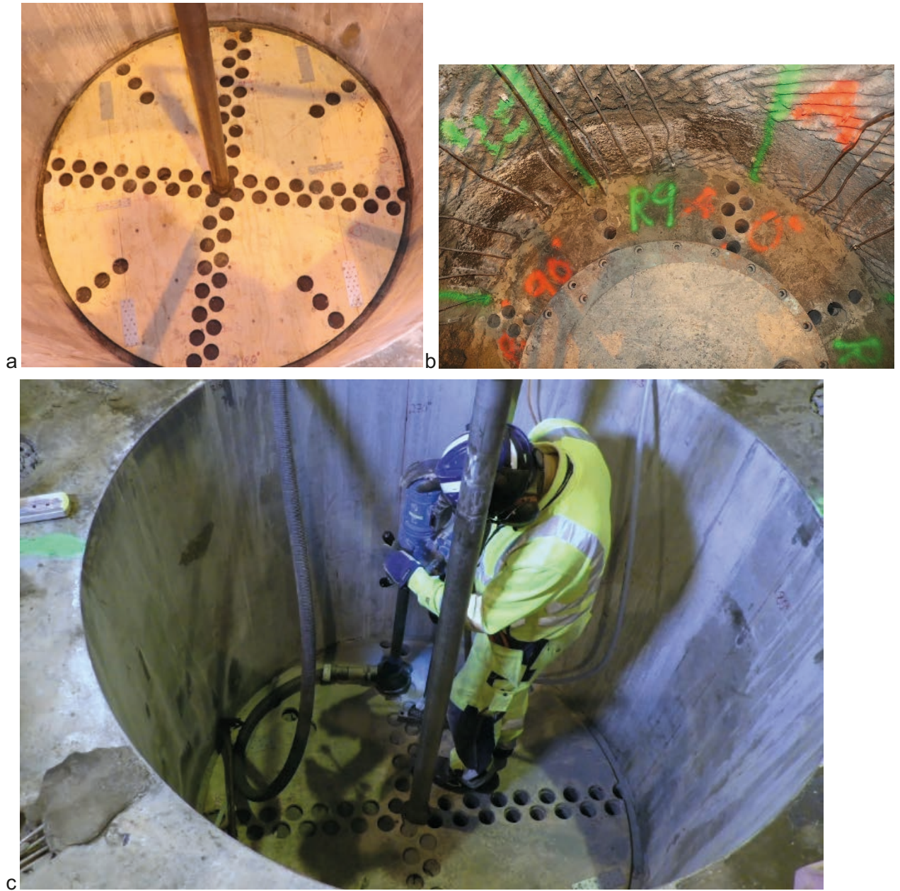
Figure 15-21. Drilling template and sampling of bentonite by core drilling. a) Drill template for complete blocks; b) Sampling of a bentonite ring; c) Drilling of samples.
