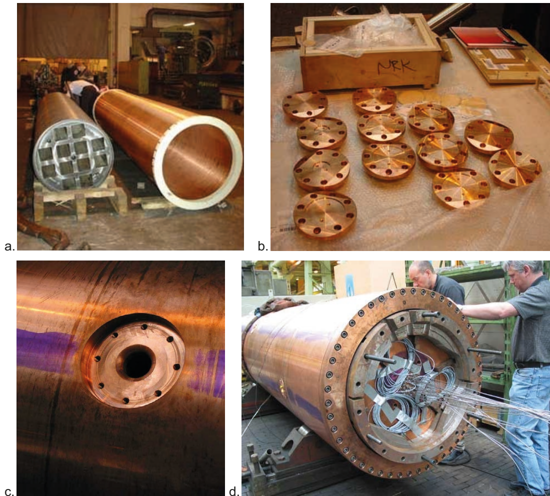
Figure 3-7. The canister as used in the Lasgit test. The canister comprised a standard KBS-3 canister, made up of a copper canister and cast-iron insert (a). Twelve filters (b) were placed at three levels along the length of the canister in recesses (c). The complete Lasgit canister is shown in (d) with the filters in place and the associated pipework coming through the canister lid.
