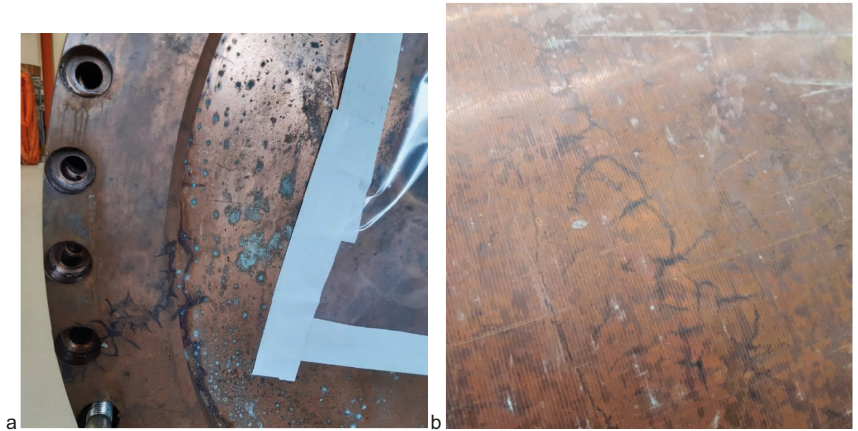
Figure 15-30. Dark brown features were seen on the surface of the canister: a) Bottom of the canister; b) Side of the canister.
