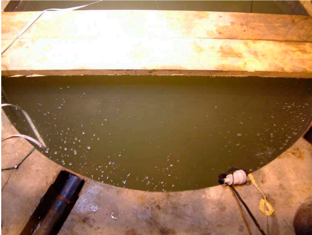
Figure 2-9. Gas bubbles on the water surface in the Lasgit hole.
