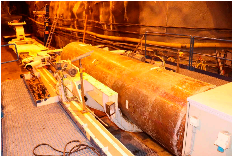
Figure 15-26. The canister removed from the deposition hole.
