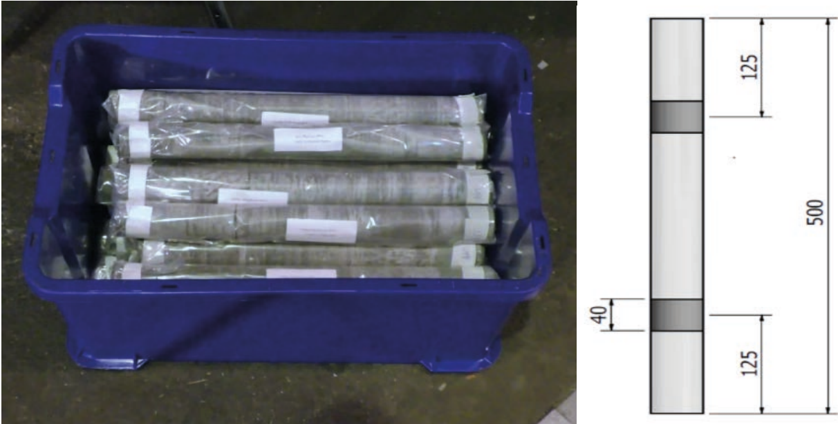
Figure 15-20. Labelled cores and position for samples to be analysed.
