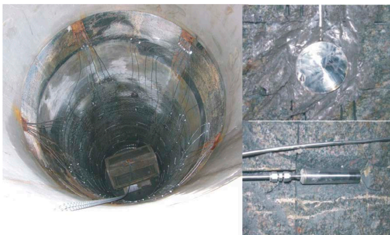
Figure 3-12. Sensors on the rock wall. The photograph on the left-hand side shows a view looking into the Lasgit deposition hole showing tube work containing the electrical connections from total stress and porewater pressure sensors mounted on the rock face. The photographs on the upper and lower right-hand show a total stress and a porewater pressure sensor respectively.
