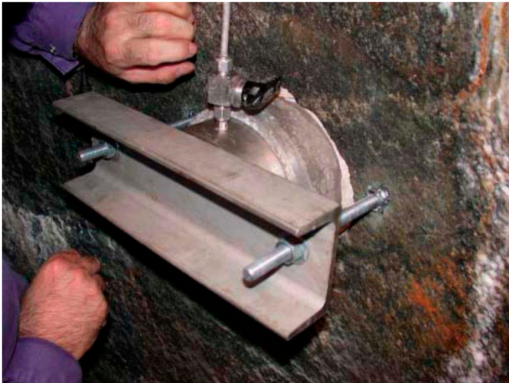
Figure 2-11. The surface packer system of BGR shown in situ ready for the start of a test.
