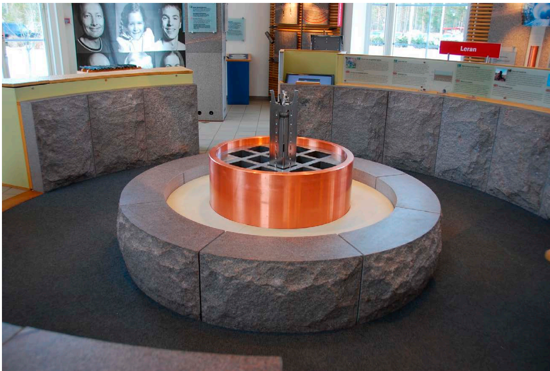
Figure 18-1. The KBS-3 disposal concept. Fuel rod assemblies are held within an iron insert, inside a copper canister. Surrounding this is pre-compacted bentonite rings isolating the canister from the crystalline wall rock.
