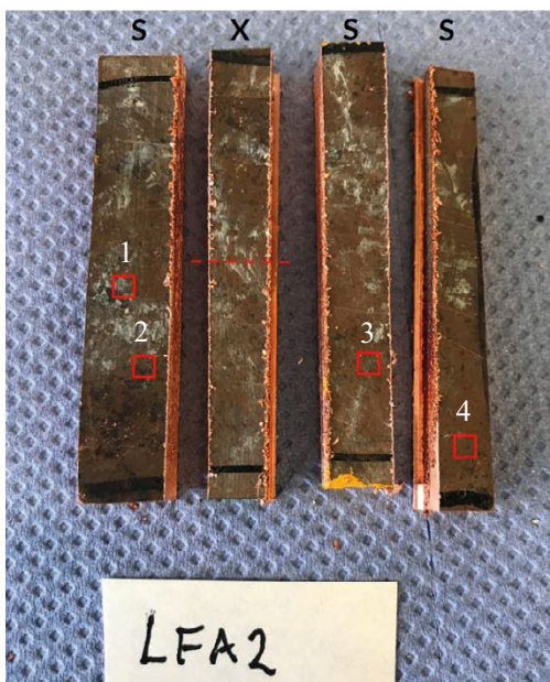
Figure 3-52. Overview of filter housing LFA2 and the area, marked with a black rectangle, of which sample coupons for analysis were to be taken.
