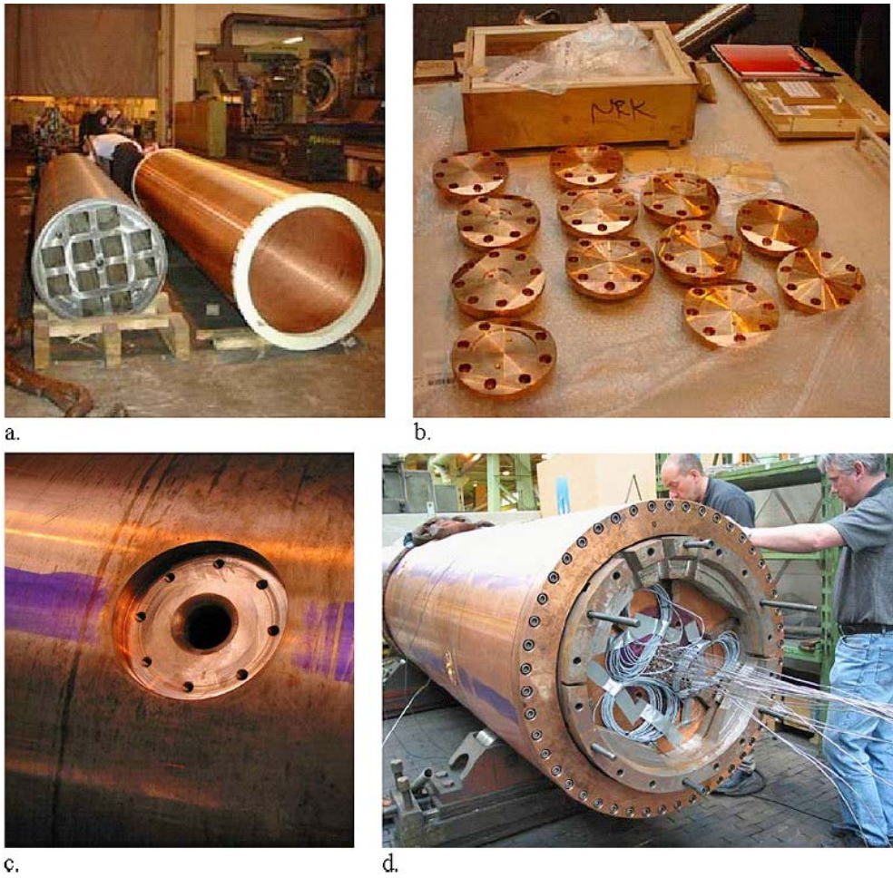
Figure 1-1. The canister used in the Lasgit experiment. A full-size canister and cast iron insert was used (a). 12 filter assemblies (b) were placed in recesses on the canister surface (c). A 13 th filter assembly was situated at the base of the canister. Filters and 45° markings along the canister are visible together with pipework through the canister lid, in the top view in (d).
