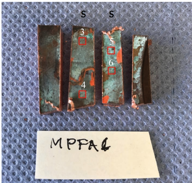
Figure 3-30. Two out of four test coupons taken from filter housing MPFA1. 'S' denotes coupons chosen for surface analysis.
