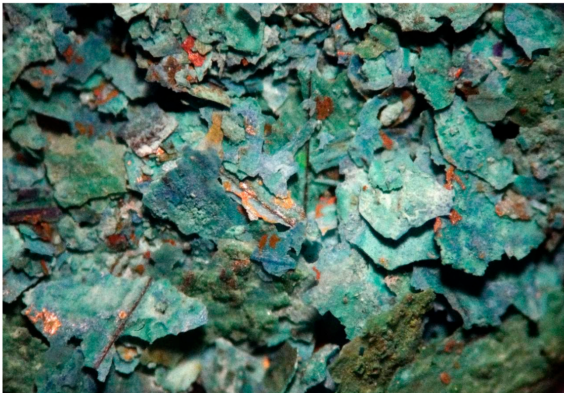
Figure 2-2. Copper corrosion products scraped from the Lasgit canister after retrieval at the Canister Laboratory. Sampling was made from the area marked with a grey rectangle in Figure 1-3c.
