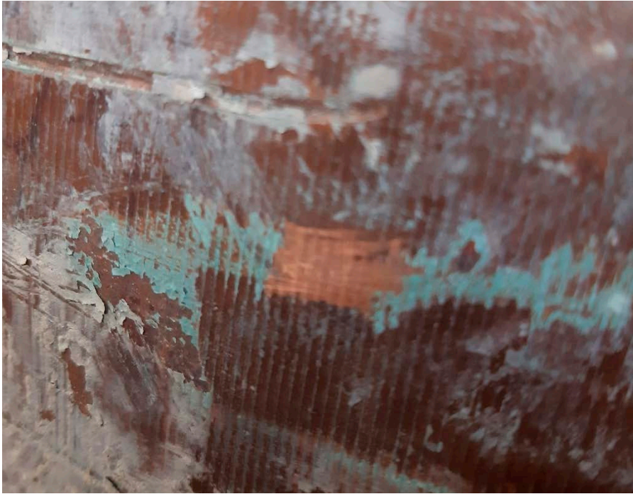
Figure 3-97. Close-up of area with green-blue deposits, of which some has been removed using a scalpel.
