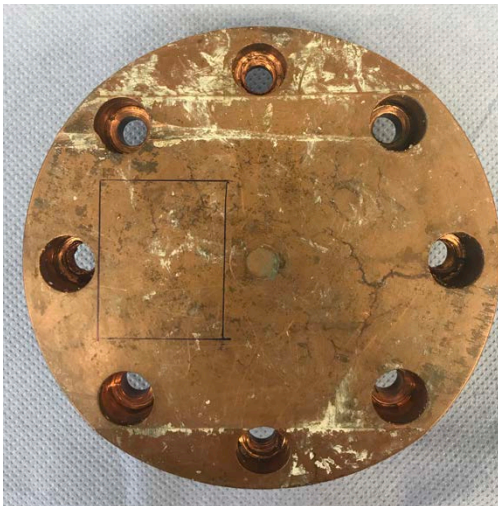
Figure 3-52. Overview of filter housing LFA2 and the area, marked with a black rectangle, of which sample coupons for analysis were to be taken.
