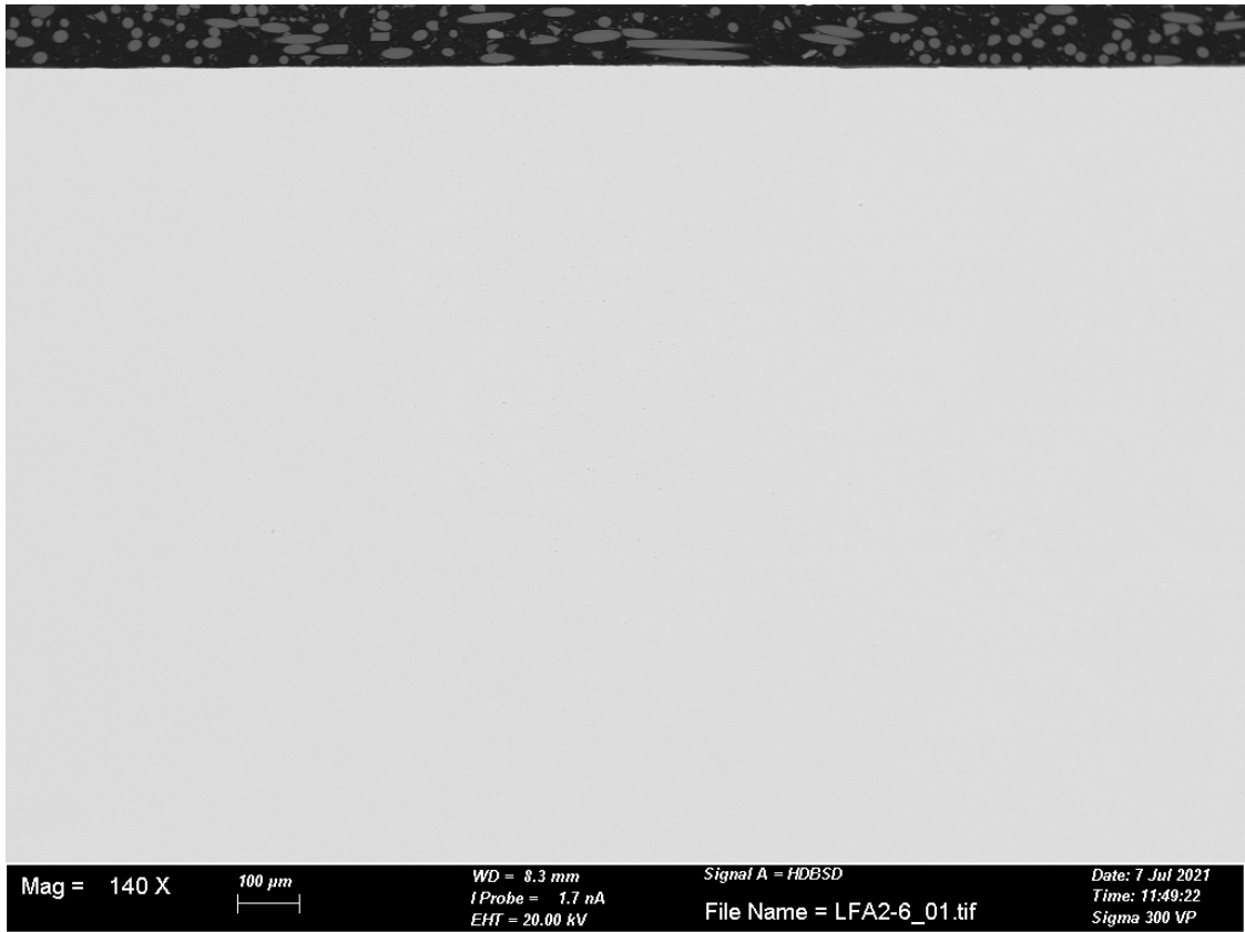
Figure 3-68. SEM image overview of cross section at \times 140 magnification, LFA2.
