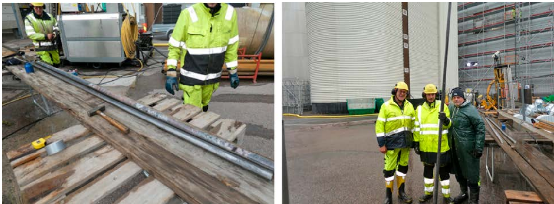
Figure 5-5. The split-tube has just been pumped out from the core barrel containing a 3 m long core with 45 mm diameter.
