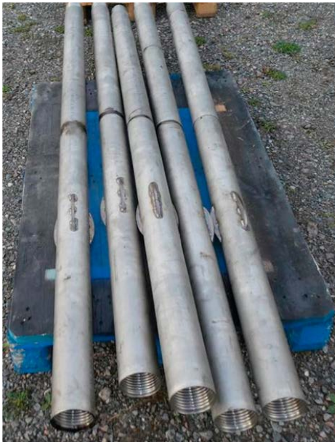
Figure 5-4. Left: As monitoring boreholes probably will be used for several decades, the inner casing is made of acid proof stainless steel. Right: The casing is lowered into the outer casing, and is centralized by three steerings for every three metres casing length.
