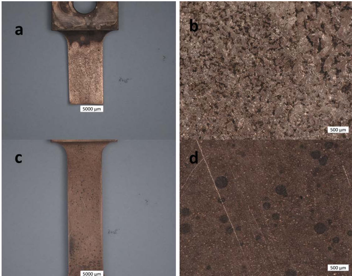
Figure 5-72. Stereo pictures of samples from experiment 3 (a and b) and experiment 6 (c and d) after the sulphide film removal.
