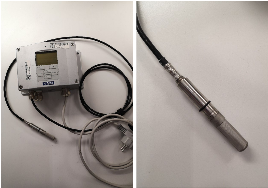
Figure 5-12. Capacitive hygrometer HMT330 (left) and the probe (right).
