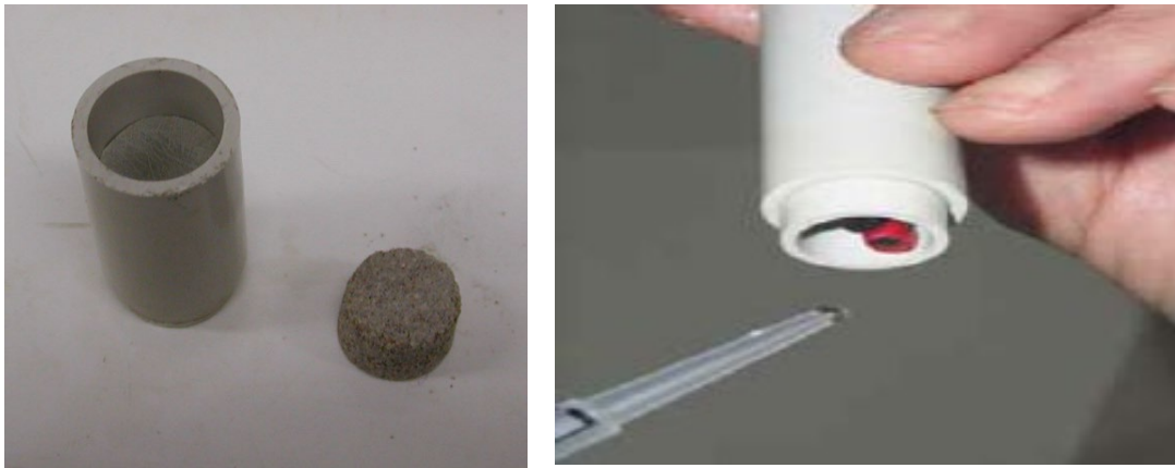
Figure 5-14. Sample and container in psychrometer of transistors (in left) and preparation of the sensor adding a tear of pure water (in right) (Hoffmann 2005).
