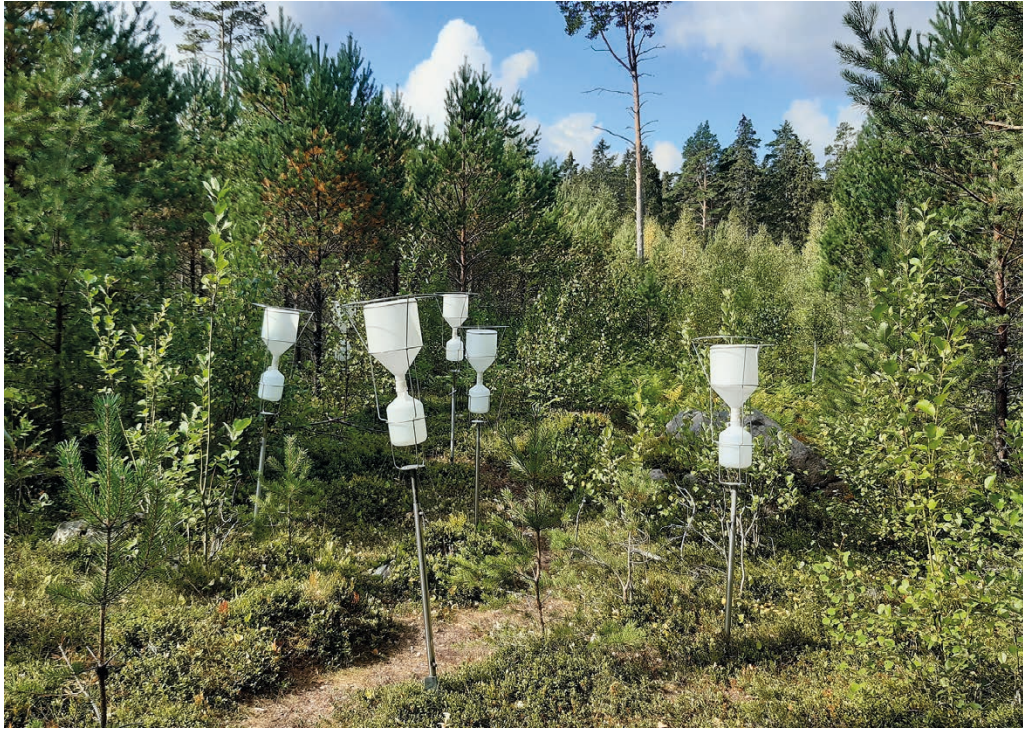
Figure 4-2. Precipitation sampler setup of six funnel-shaped polyethylene containers (summer type) at location PFM008126.
