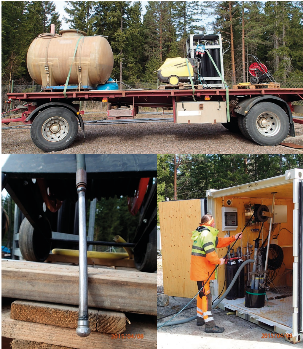
Figure 2-2. Cleaning equipment used to clean the standpipes prior to pumping and sampling.
