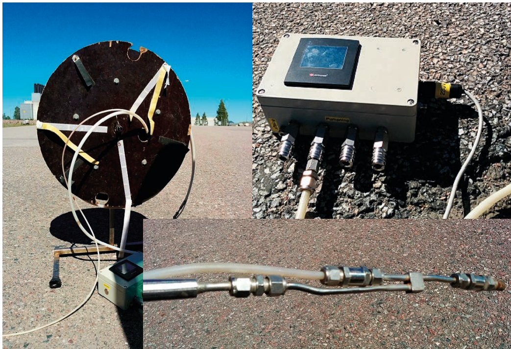
Figure 2-5. The equipment used for gas-lift pumping. On the left, the tubing lowered down the standpipe (the narrower tube for sample water and the wider for gas) on a bobbin to simplify the lowering. To the upper right the control unit for the pumping/gas supply and lower right the end of the gas-lift pump.
