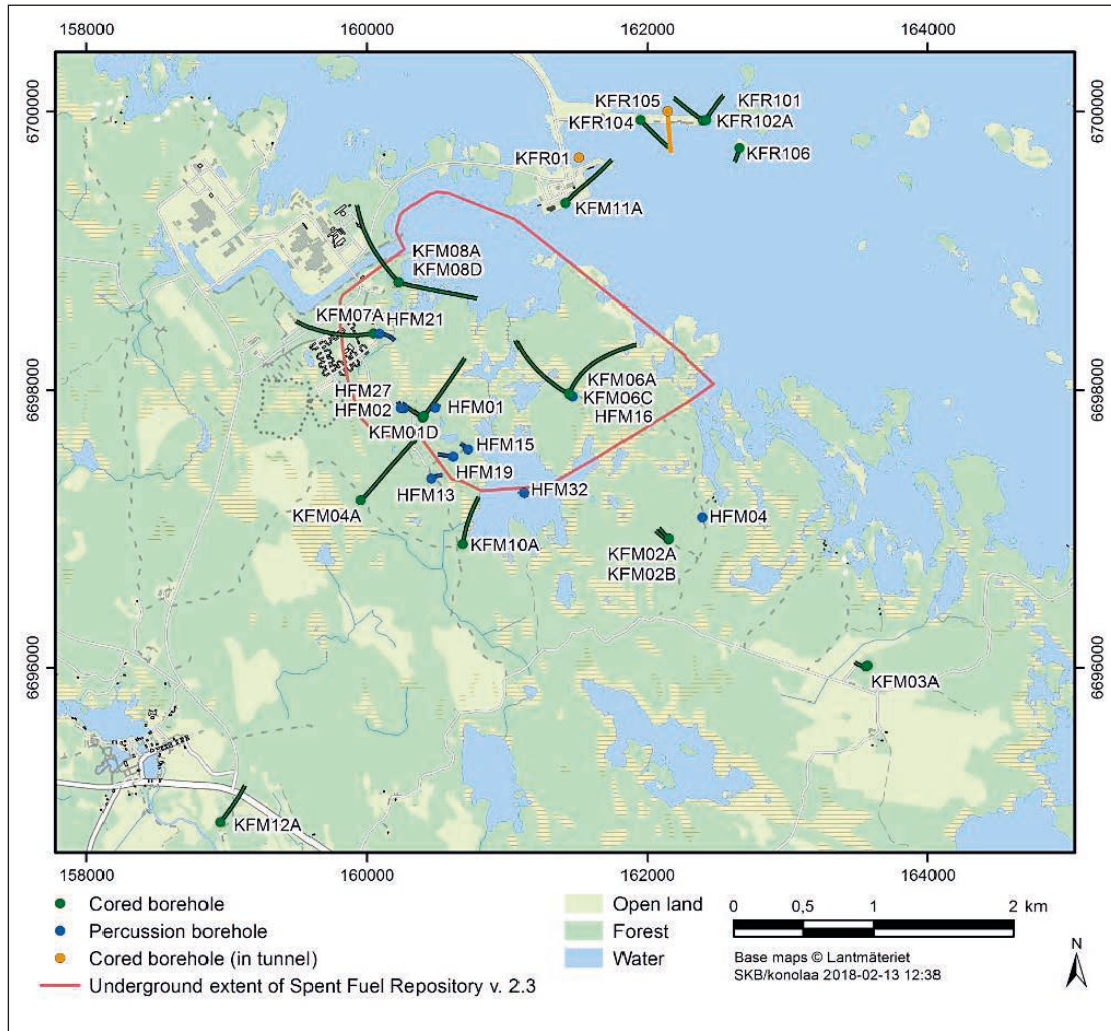
Figure 1-1. General overview of the Forsmark area and the boreholes included in the hydrochemical monitoring program for groundwater. The (telescopic) cored boreholes and the percussion boreholes within the monitoring program are marked with green and blue filled circles, respectively. Tunnel boreholes are marked with orange filled circles.
