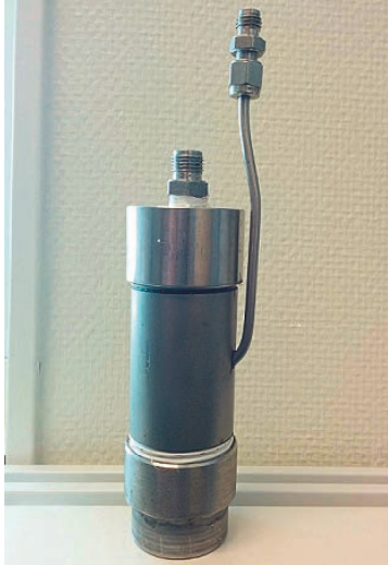
Figure 2-4. The docking unit, which is used together with the pump (GEOPUMP UV-45). Instead of using the mini-packer to isolate the lower part of the standpipe with the pump, the unit is tightly fitted to the tube in the bottom of the standpipe. The photo shows the docking unit used in normally equipped boreholes. The one used in KFM08D is modified to match with the special equipment in PEEK, but is very similar to the one in the photo.
