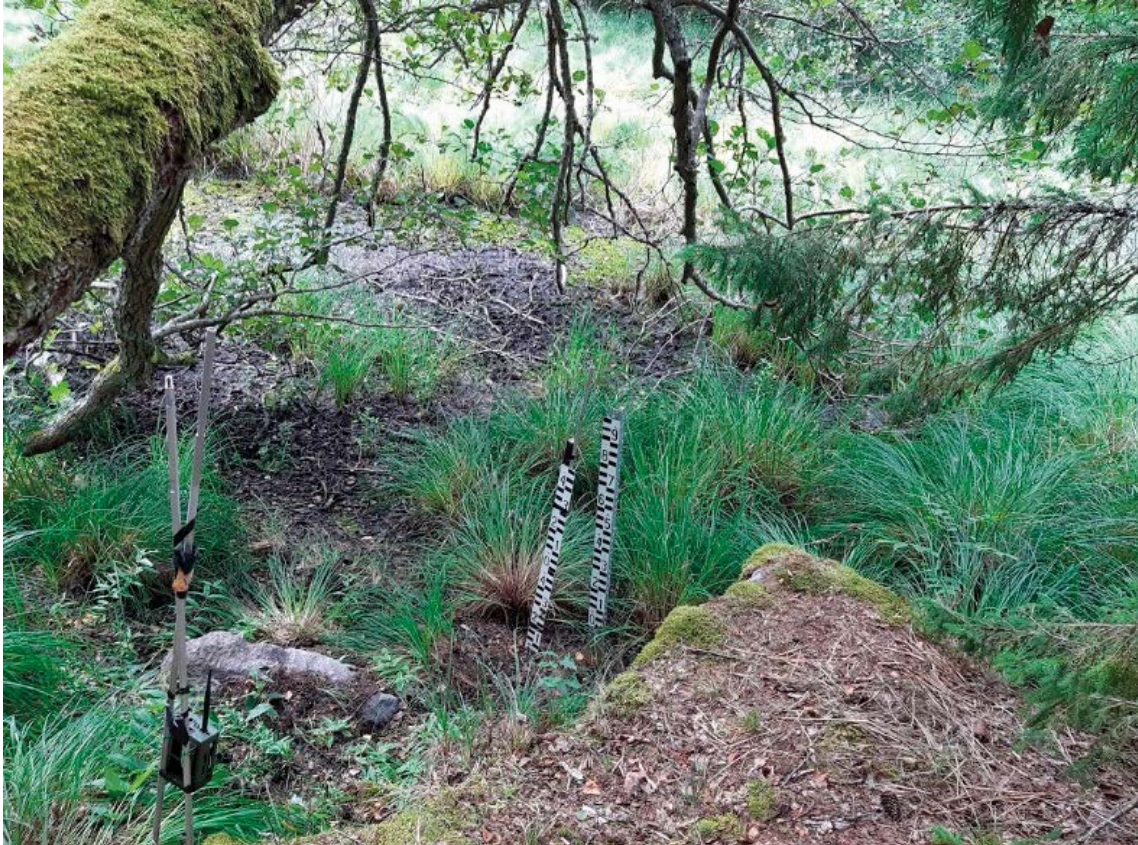
Figure 4-3. Photo of the wildlife camera (PFM008098, left), the gauging scale PFM008262 (middle) and the supplementary gauging scale PFM008263 (right) in pond 122.
