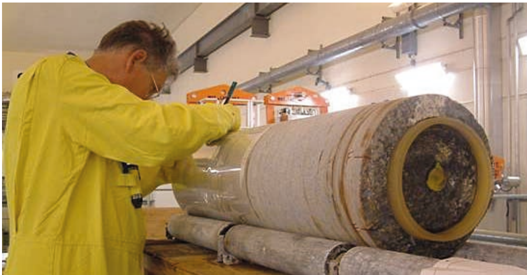
Figure 3-6. Mapping fracture traces on core.
