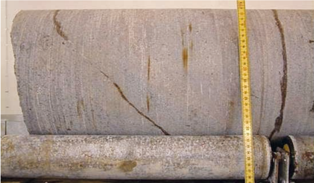
Figure 3-14. Drill core with open fractures at 60 cm and 80 cm (dark streaks, caused by moist) from the right hand side. Core rotated to position F.
