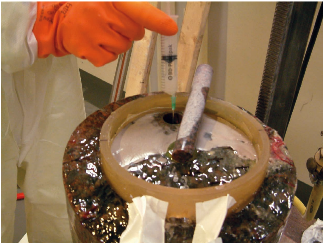
Figure A12-4. Drill hole of sample A-16 is emptied from drilling water, before plugged by rubber cork.
