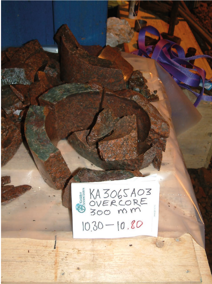
Figure A7-15. The over-core of drill phase 1, chainage 10.3 to 10.8 m. Core pieces are joined to re-create a hollow cylinder. The fracture at 10.74 m, ending the core, is facing upwards.
