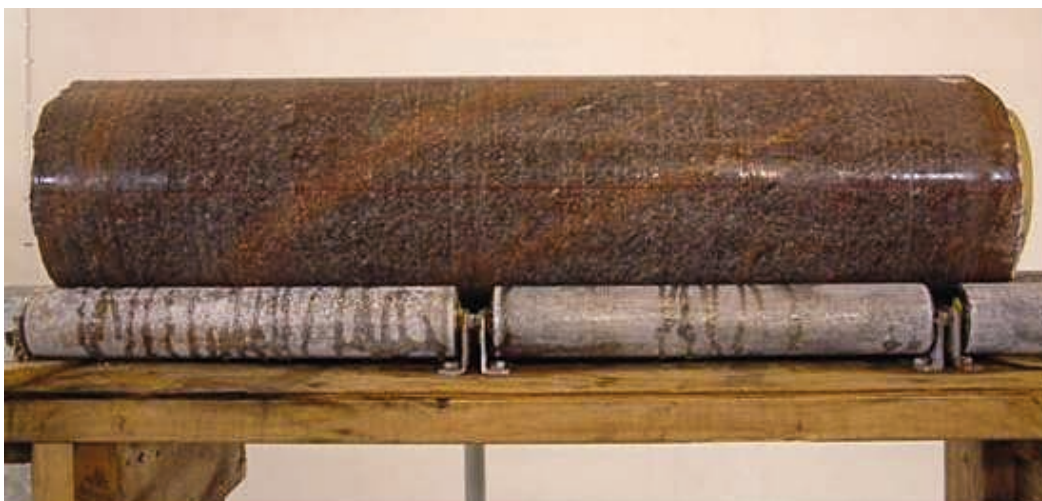
Figure 3-7. Drill core rotated to position A (chainage line) facing camera lens. Rock is a so-called Ävrö granite with a diffuse foliation or lineation. Reddish miscolouring is aligned with fractures sealed with quartz or another hard mineral.
