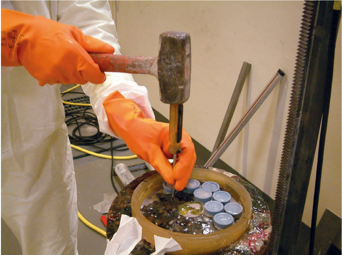
Figure A12-5. Core breaking and retrieval of sample A-4. Drill holes of samples A-12, 6, 5, 10, 18, 11, and A-17 are plugged by rubber corks.
