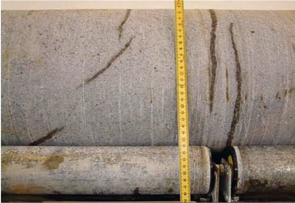
Figure 3-16. Drill core with open, discontinuous fractures at 60 cm and 80 cm (dark streaks, caused by moist) from the right-hand side. Core rotated to position B, detail.
