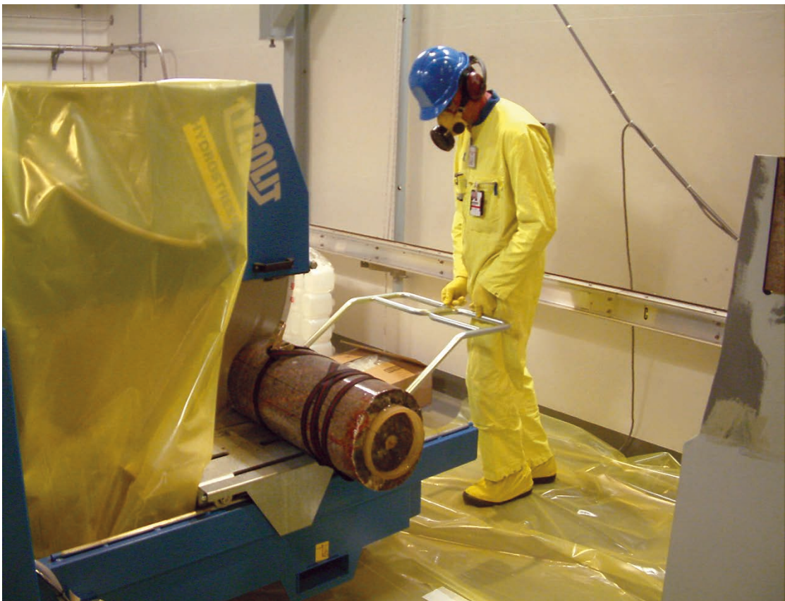
Figure 4-5. Cutting of the core.
