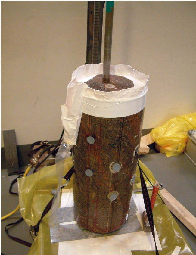
Figure A12-6. Drilling of a C-core sample.
