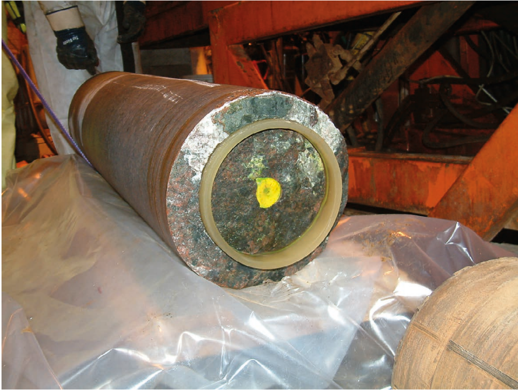
Figure A7-20. Over-core 10.74 m to 11.82 m. Target fracture at 10.74 m with the 177 mm diameter core stub inside the cylindrical PU sealing, where radionuclide tracers were circulated.
