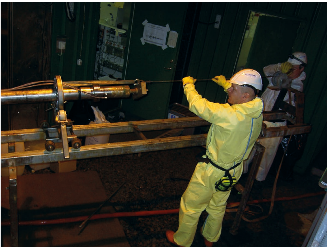
Figure A6-4. First phase of hauling is coming to final. Special protective clothing is used due to potential risk of contamination from radionuclides used in the experiment.
