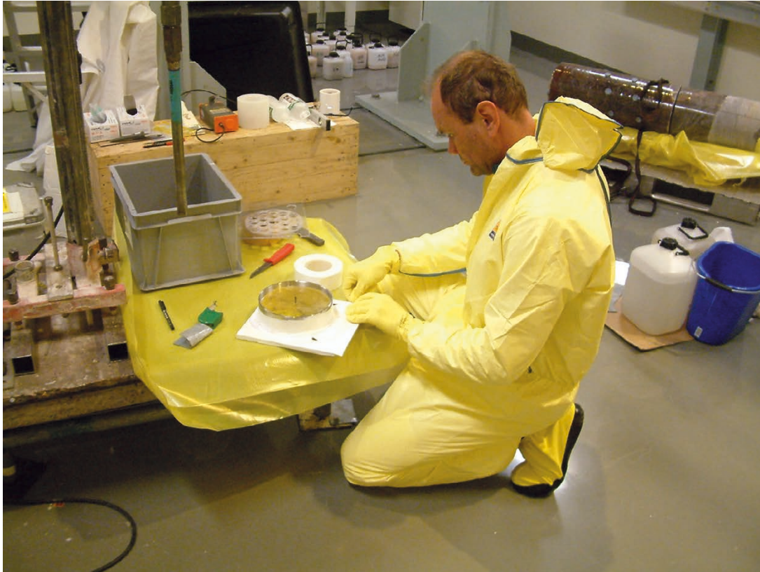
Figure A14-3. PEEK lid with (injected) yellow marked epoxy and protective coating of colourless epoxy is fastened to a stiff plate before drilling of the B-core samples.
