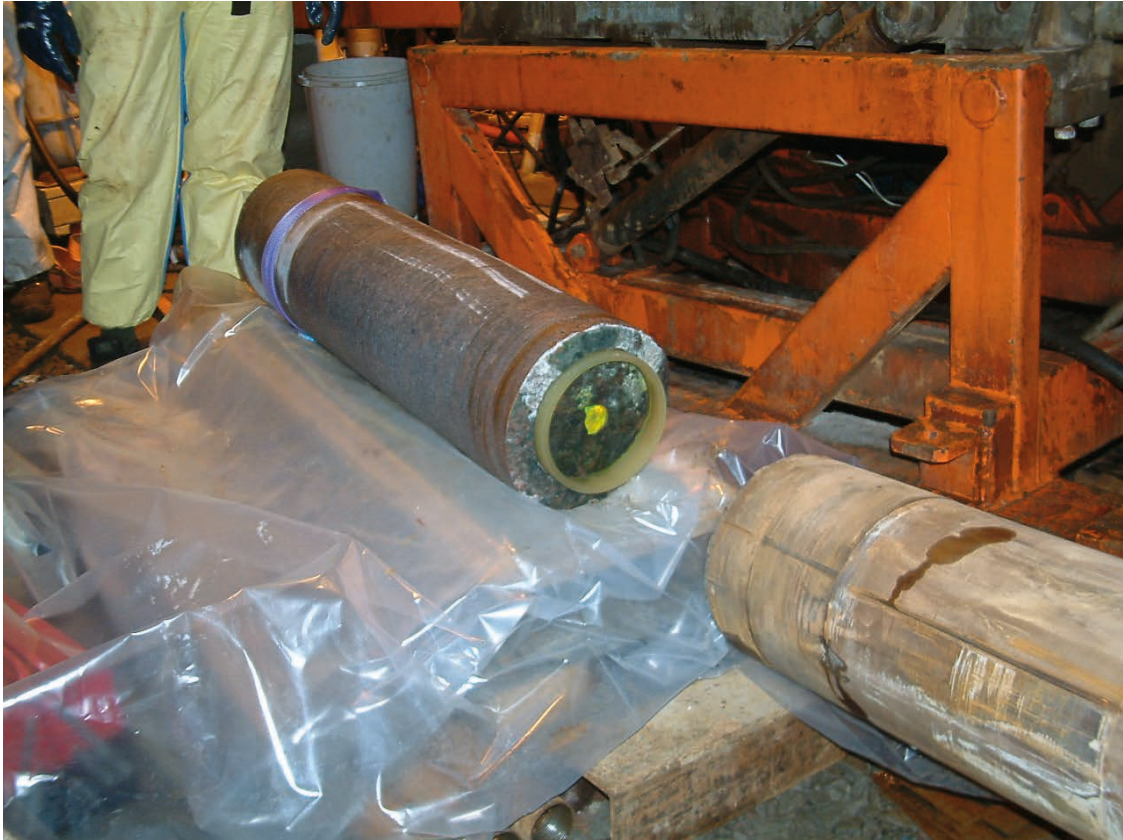
Figure 2-13. One piece, 278 mm diameter, 10.74–11.82 m core retrieved from over-core drilling of borehole KA3065A03. Target fracture with the 177 mm diameter core stub inside the cylindrical PU sealing where radionuclide tracers were circulated.
