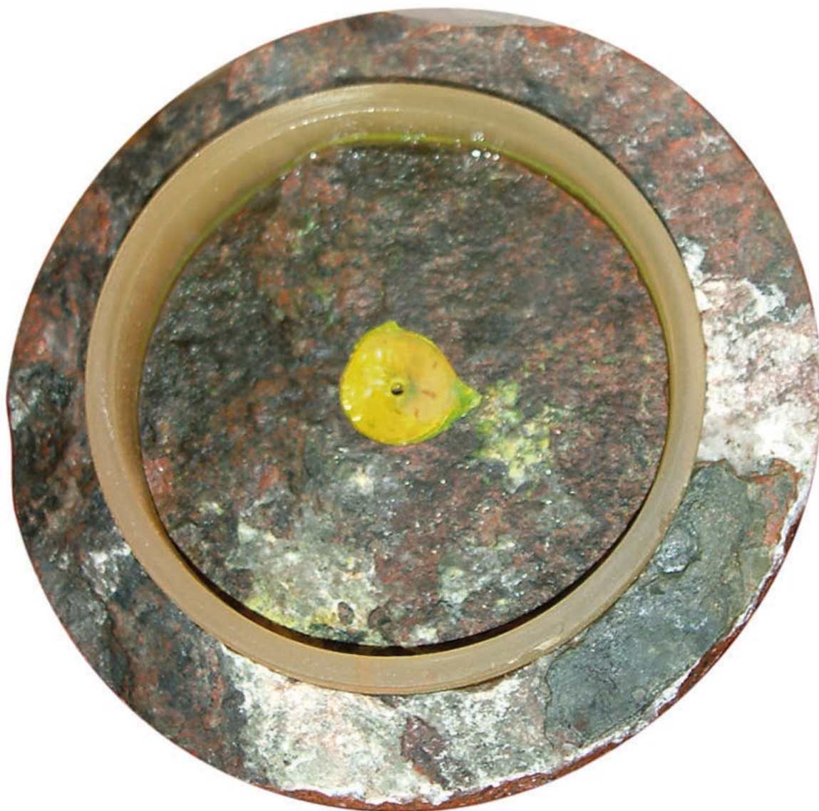
Figure A11-1. Target fracture at 10.74 m with the 177 mm diameter core stub inside the cylindrical PU sealing. The core is rotated to show the orientation in the borehole, i.e. the core low side is down. The photo is taken immediately after core extraction at the experimental site NASA3067A in the Äspö HRL, cf Figure A7-20.
