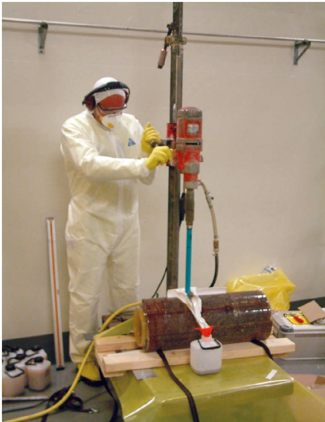
Figure 4-6. Drilling of a D core sample.
