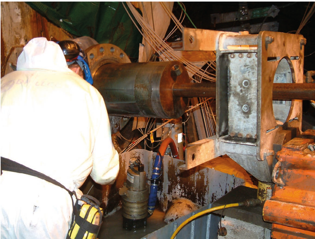
Figure A7-8. Core barrel coming out of borehole.
