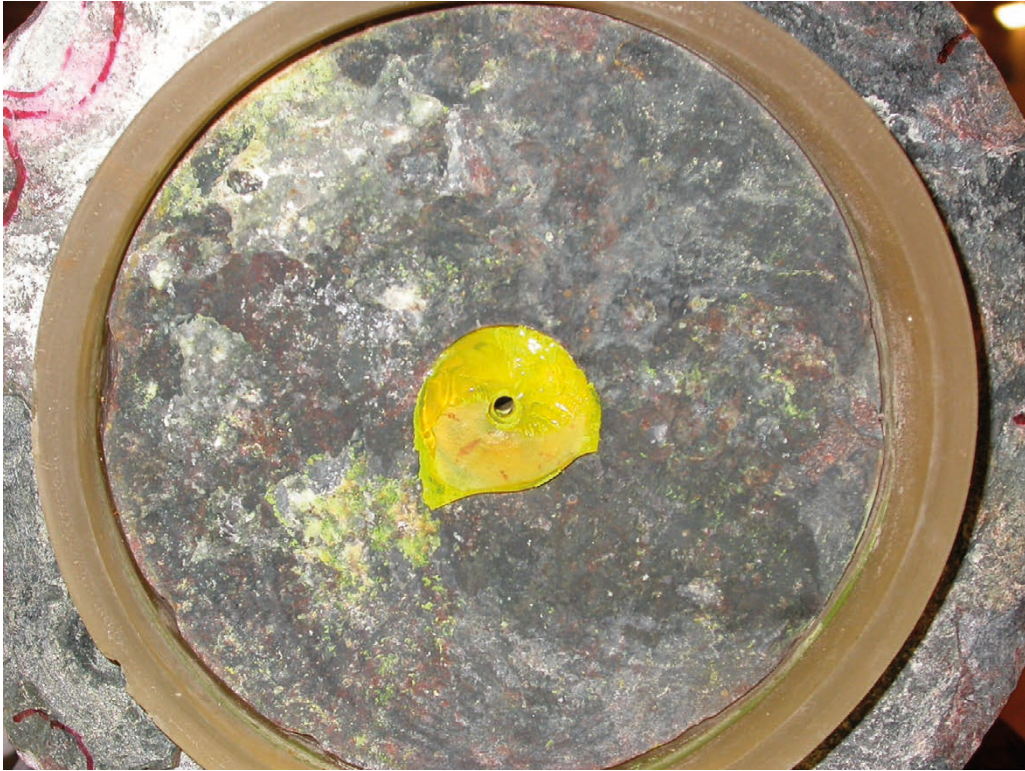
Figure A11-3. Target fracture at 10.74 m with the 177 mm diameter core stub inside the cylindrical PU sealing. The photo is taken at Clab in connection with the first marking of the core. See Section 3.1. Remains of the loosened yellow epoxy resin can be seen on the fracture surface.
