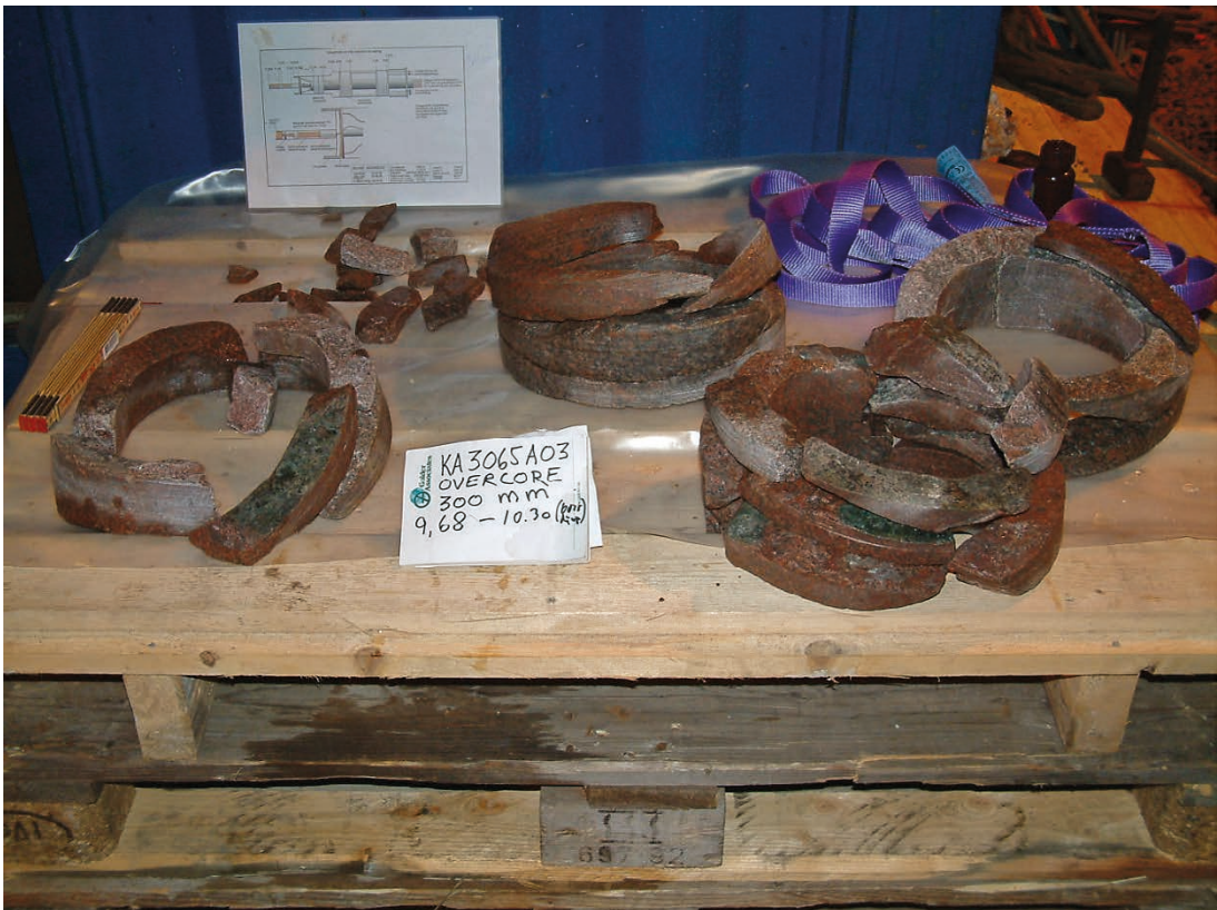
Figure A7-10. The over-core of drill phase 1, chainage 9.68 to 10.3 m. Core pieces are joined to re-create a hollow cylinder.
