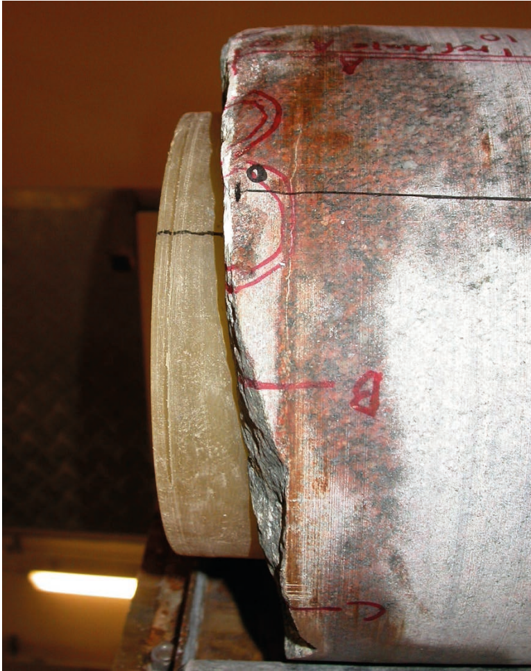
Figure 4-2. New length reference chainage zero (scaling 2007-06-08), based on position of borehole equipment in the 36 mm diameter extension borehole. The black line marks the lower side of the core, as it was oriented in the rock during the in situ experiment. The end mark of this line next to the black “0” on the stub marks the new length reference chainage.
