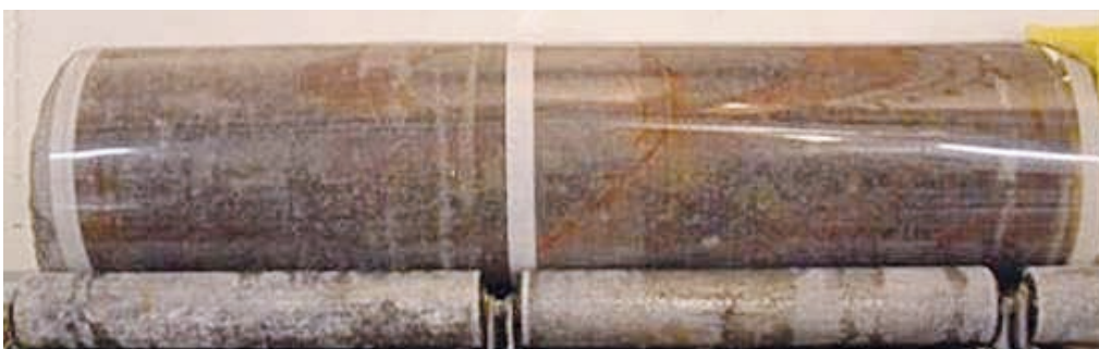
Figure 3-18. Core rotated to position C. Sealed fracture traces marked in red.
