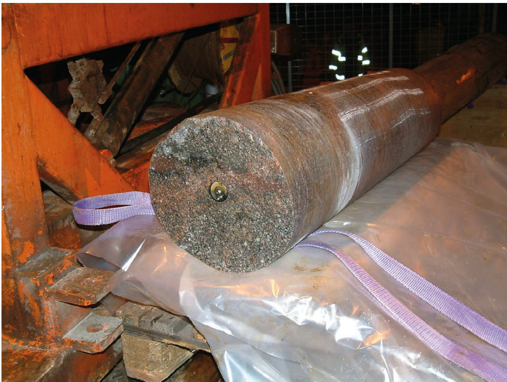
Figure A7-21. Over-core 10.74 m to 11.82 m. Breached end at 11.82 m, 36 mm borehole with parts of the special packer used to restrict the slim hole test section is seen in centre of core.
