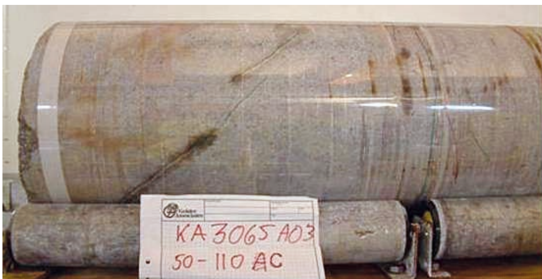
Figure 3-9. Down part of core 50–110 cm rotated to position C, showing that the open fracture at 80 cm with 45^\circ to core axis is not continuous.
