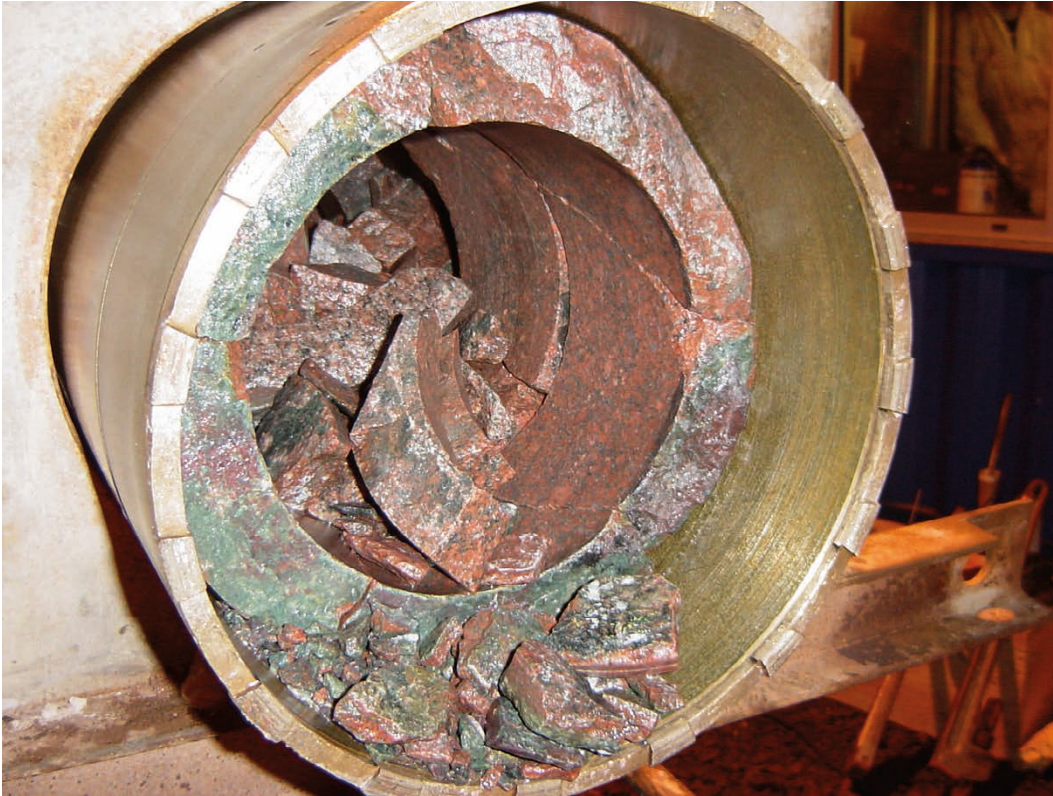
Figure A7-11. Core retrieval of drill phase 1, chainage 10.3 to 10.8 m. Fracture at 10.74 m, facing towards the drill bit, is ending the core.
