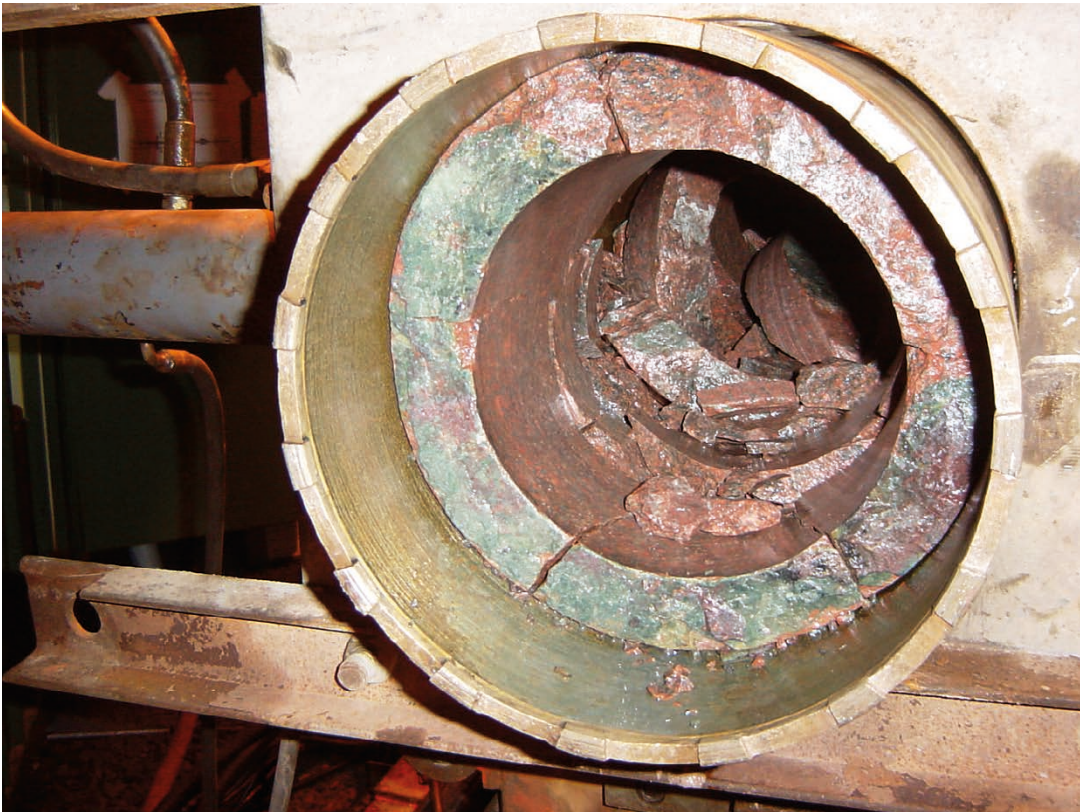
Figure A7-12. Core retrieval of drill phase 1, chainage 10.3 to 10.8 m. Fracture at 10.74 m, facing towards the drill bit, is ending the core. Cf Figure A7-11, photo from another visual angle.
