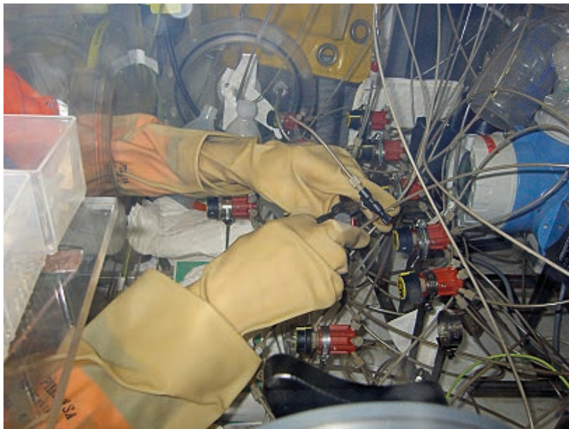
Figure A6-1. Disconnecting circulation tubes in glove box in experimental container (C1) before removal and dismantling of borehole equipment.
