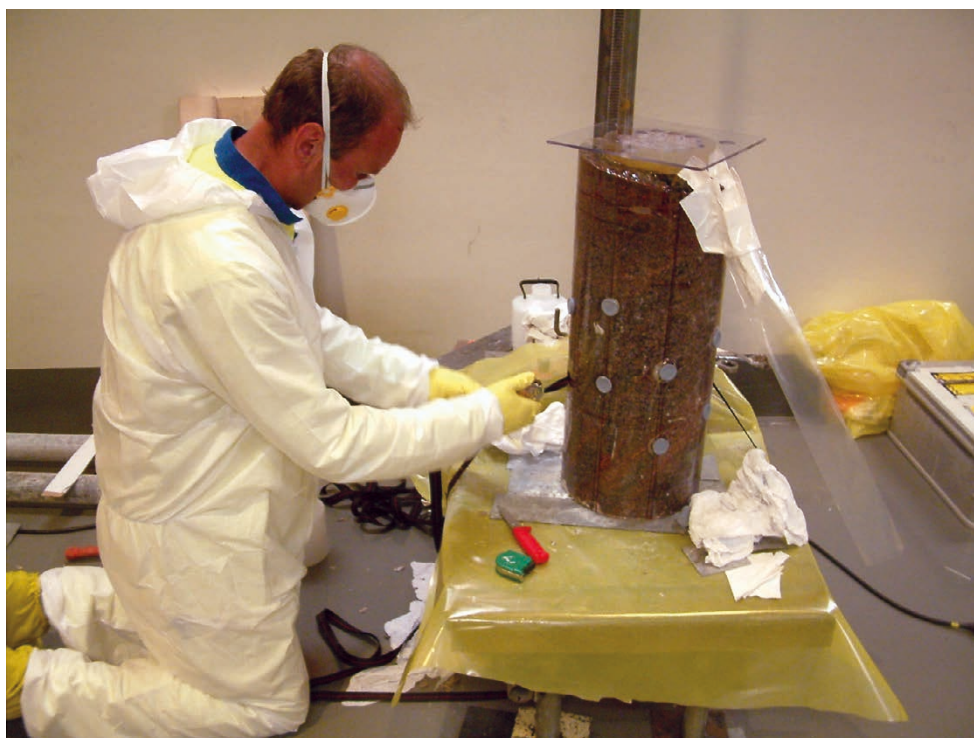
Figure A12-2. Fastening of over-core before drilling of A-core samples.
