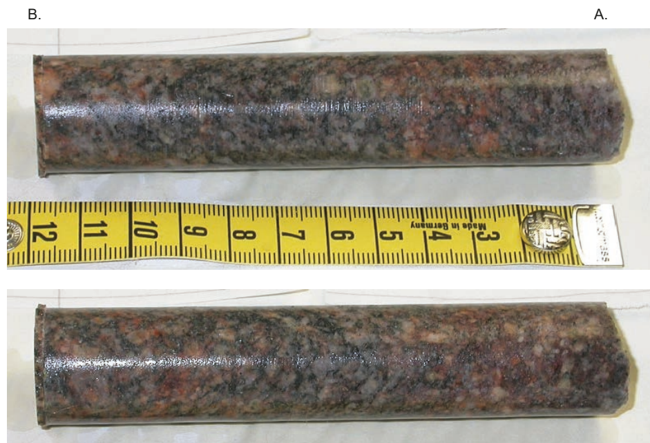
Rock core D4 with orientation 0°–180° (upper picture) as well as orientation 180°–360° (lower picture).
