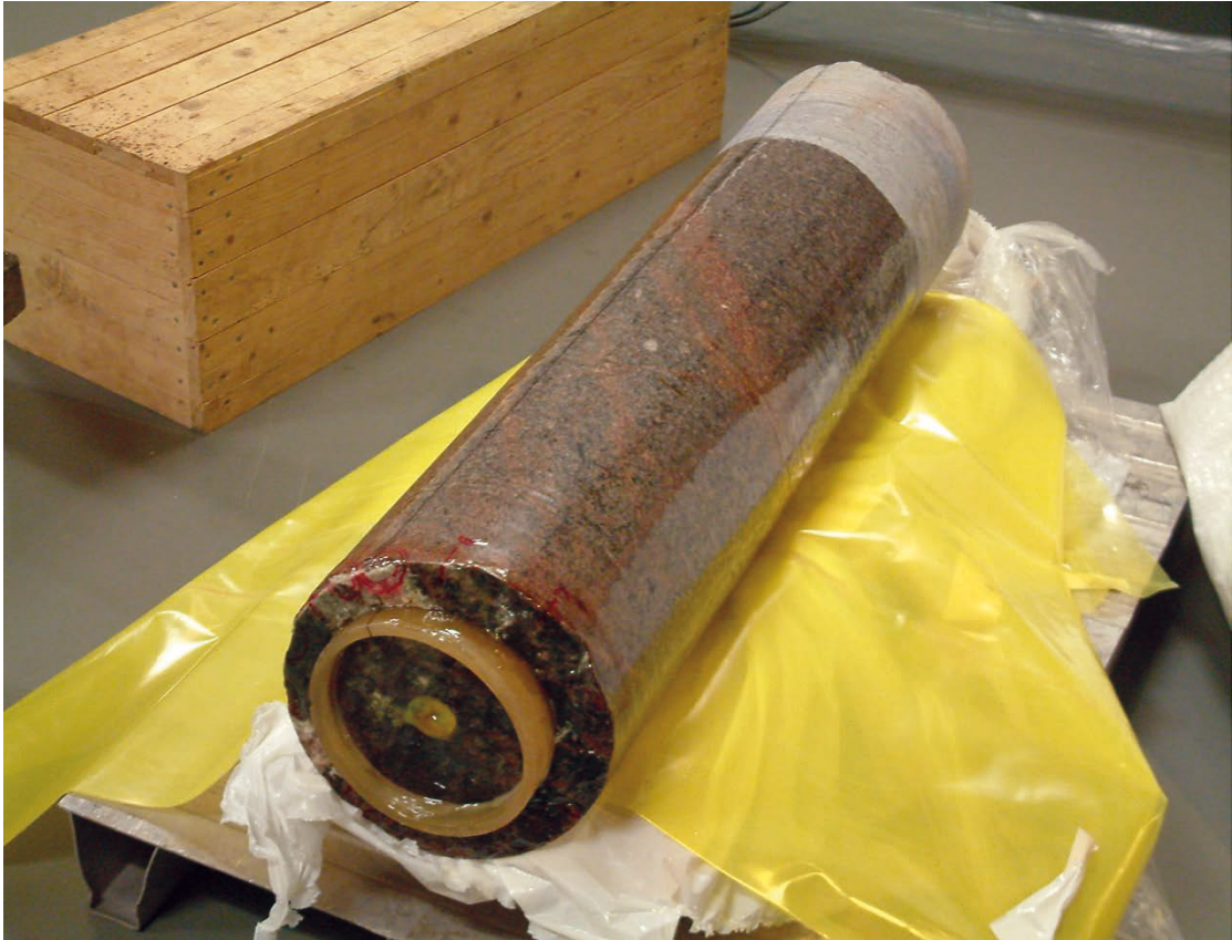
Figure 4-4. The Epoxy coated 278 mm diameter core before cutting.
