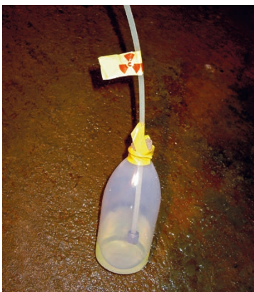
Figure 2-6. Mixture of isopropyl alcohol and yellow coloured epoxy resin collected at KA3065A03 outlet tube during epoxy resin injection.
