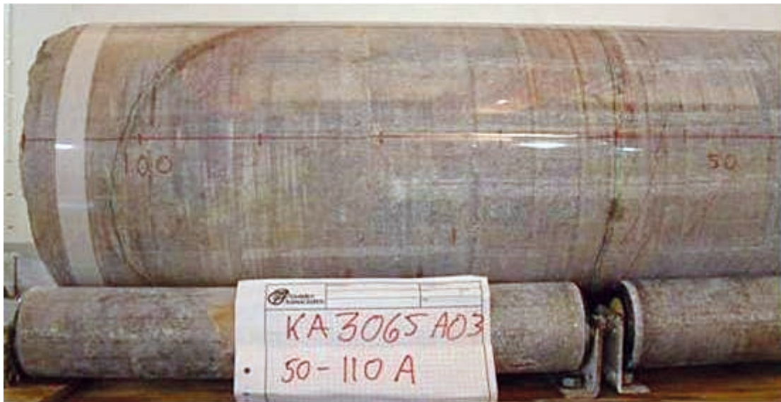
Figure 3-8. Down part of core 50–110 cm rotated to position A. Two traces of open fractures are marked with green and three short sealed fractures marked with red. The open fracture at 60 cm intersects the core with an angle of 90^\circ , and the other at 80 cm has an angle with core axis of 45^\circ .
