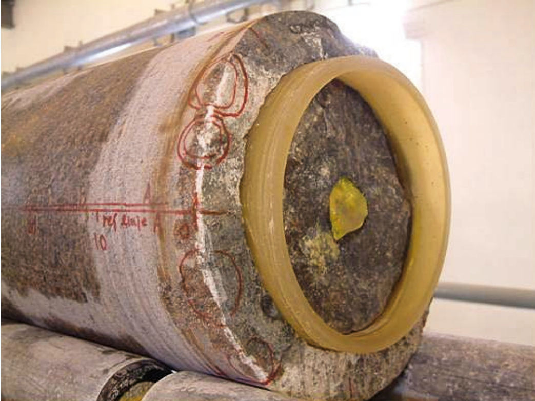
Figure 3-3. Upper end of core with PU cylindrical sealing and epoxy filled 36 mm pilot centre hole.
