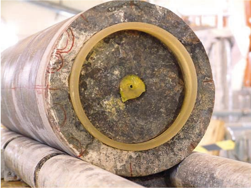
Figure 3-4. Pinch bar marks highlighted on upper end of core. Double rings indicate probable marks, single rings indicate uncertain marks.
