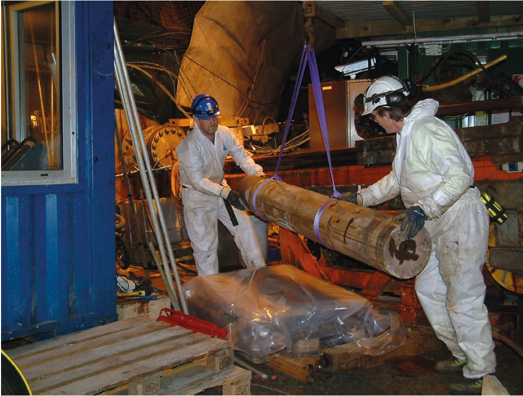
Figure A7-18. Core barrel containing retrieved core from drill phase 2 is removed from the drilling machine.
