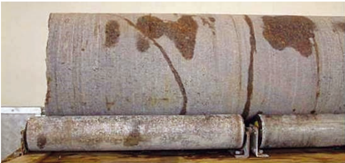
Figure 3-13. Drill core with open, continuously looking (which they are not) fractures at 60 cm (left of centre) and 80 cm (right of centre) from the upper core end. Core rotated to position G.
