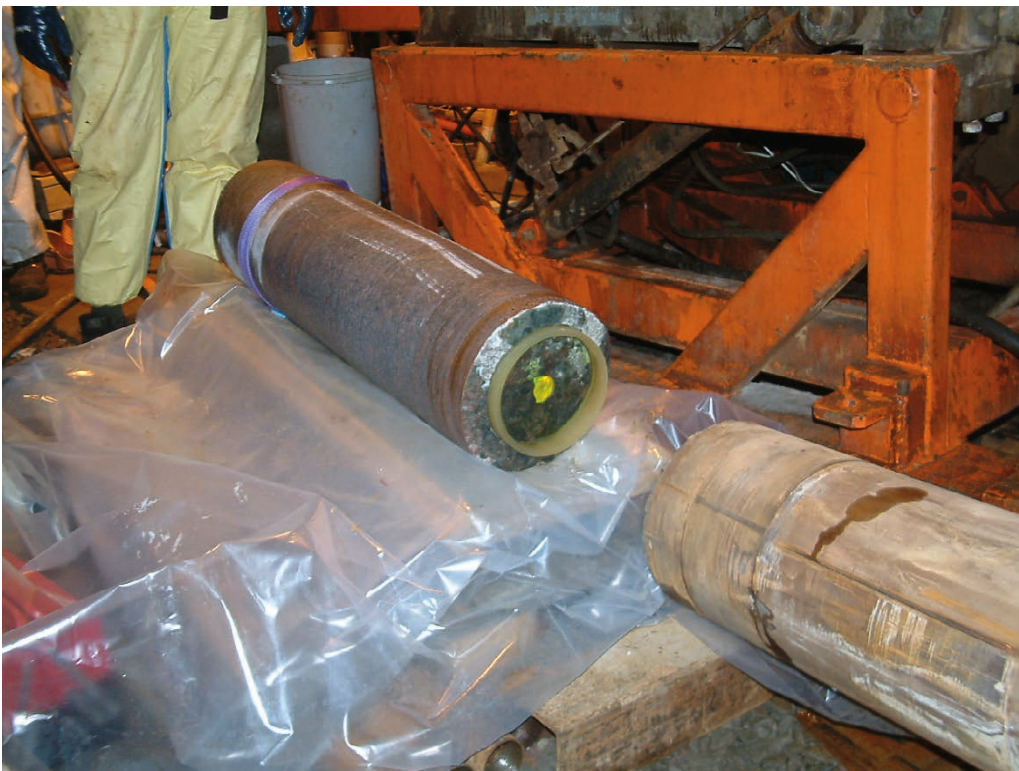
Figure A7-19. Over-core 10.74 m to 11.82 m pulled out of core barrel. Target fracture at 10.74 m is facing towards the core barrel.
