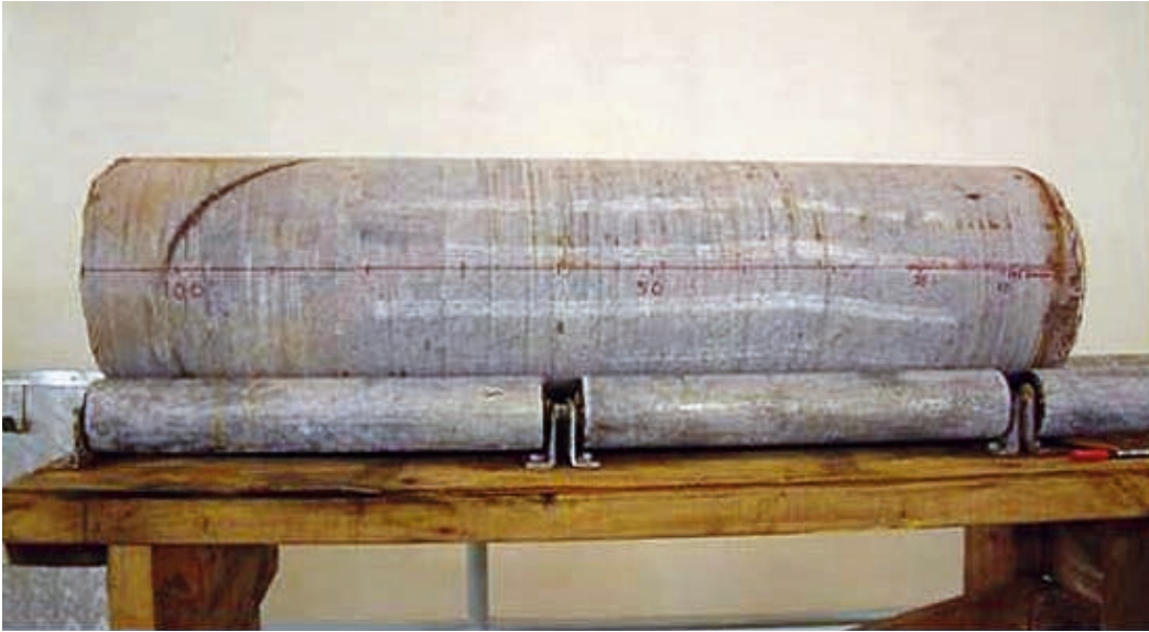
Figure 3-2. Drill core with chainage markings.
