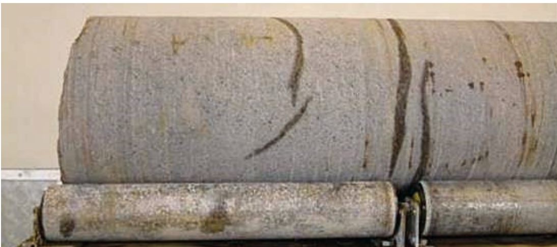
Figure 3-15. Drill core with open, discontinuous fractures at 60 cm and 80 cm (dark streaks, caused by moist) from the right hand side. Core rotated to position C.
