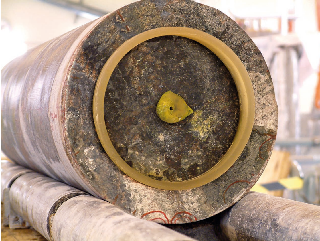
Figure A11-2. Target fracture at 10.74 m with the 177 mm diameter core stub inside the cylindrical PU sealing. The core is rotated to show the orientation in the borehole, i.e the core low side is down. The photo is taken at Clab in connection with the first marking of the core. See Section 3.1 and Figure 3-4.
