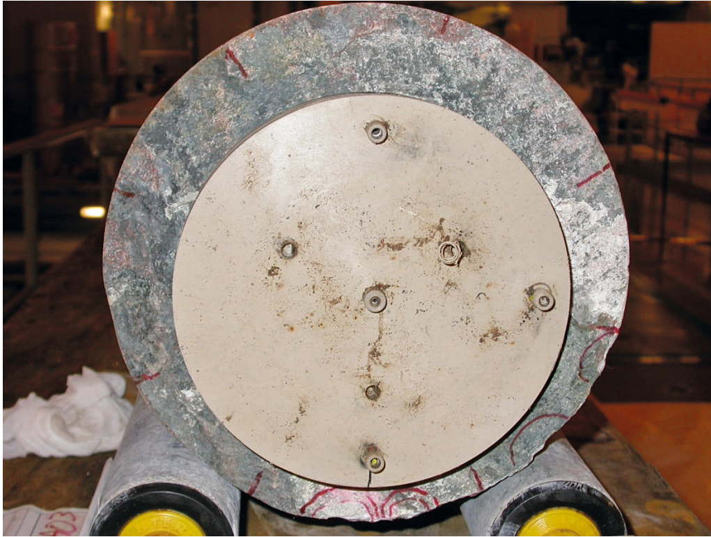
Figure 4-1. The PEEK lid matched to the fracture surface on the core stub. The core and PEEK lid having same orientation as in the borehole KA3065A03 during the in situ experiment. The eccentricity of over-core relative core stub is 4.5 mm but the angle of the view makes it look larger.
