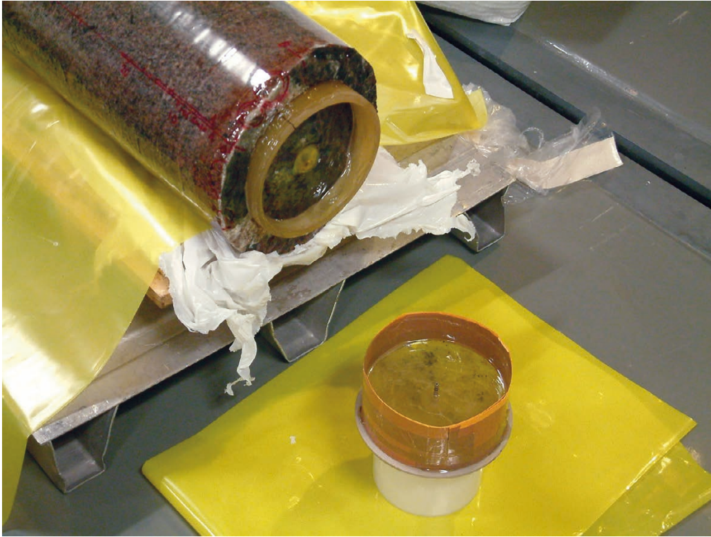
Figure A14-1. Protective colourless epoxy (EpoTec 302) cast on top of yellow marked epoxy and PEEK lid.
