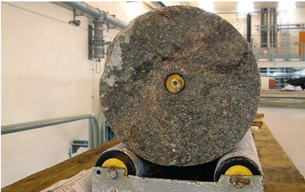
Figure 3-5. Induced breakage of down end of drill core also showing the 36 mm extension hole filled with equipment for sealing test section.
