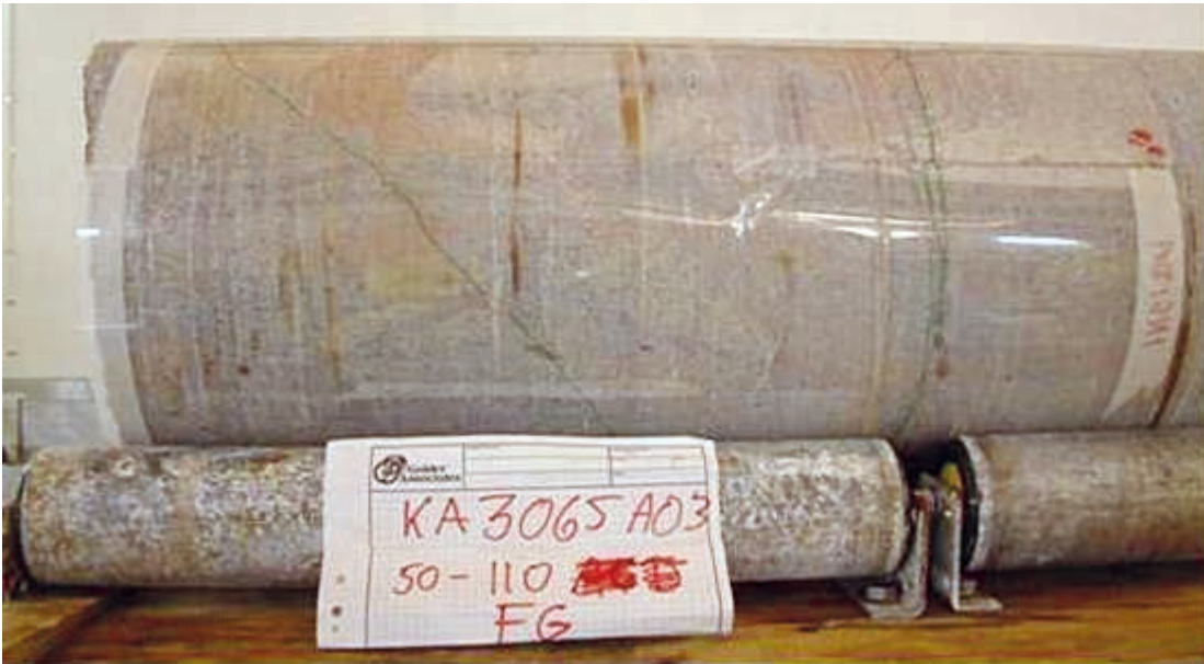
Figure 3-11. Down part of core 50–110 cm rotated to position between F and G, showing that the open fracture at 60 cm with 90° to core axis is also not continuous.
