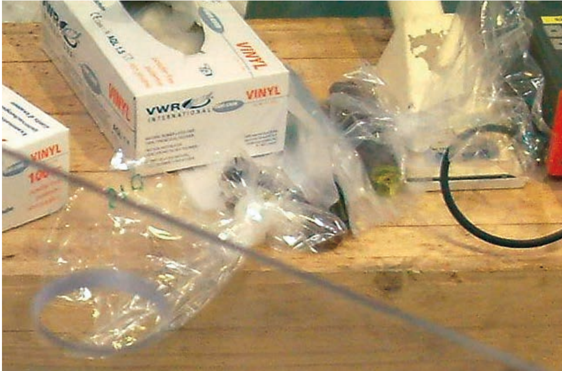
Figure A9-1. Rock core samples contained in thin plastic bags, mainly to avoid cross-contamination during cutting, drilling and storage of rock core samples. Plastic bags were not primarily used to prevent drying of the pore water and air was not evacuated from them during storage.
