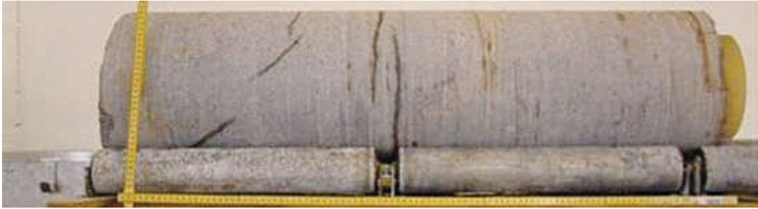
Figure 3-12. Drill core with open, discontinuous fractures at 60 cm and 80 cm (dark streaks, caused by moist) from the right hand side. Core rotated to position B.
