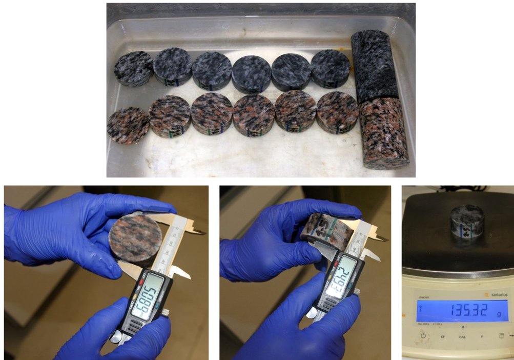
Figure 2-4. Sliced samples immersed in tap water (top) and assessment of sample size and weight (bottom).
