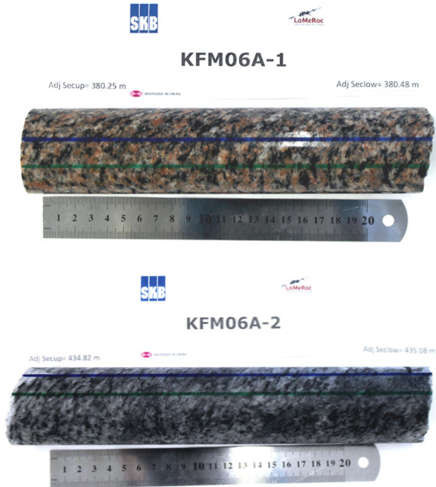
Figure 2-1. Drill cores as received: KFM06A-1 on the top and KFM06A-2 on the bottom. The cores are oriented in the pictures with their left side pointing towards the shallowest depth ( Adj Secup ). The relative location of the blue and green lines facilitates the orientation of the samples.
