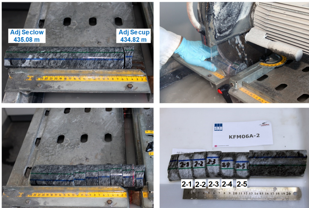
Figure 2-3. Cutting sequence of drill core KFM06A-2 for fracture toughness sample testing.
