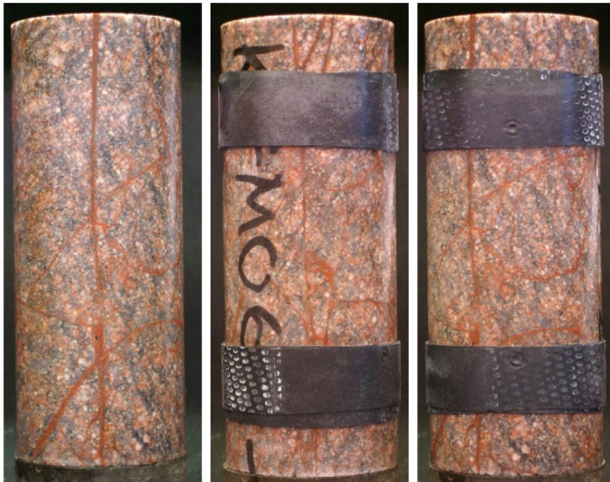
Figure 4-5. Example of a core sample with sealed fracture network tested for uniaxial compressive strength (Jacobsson 2007).
