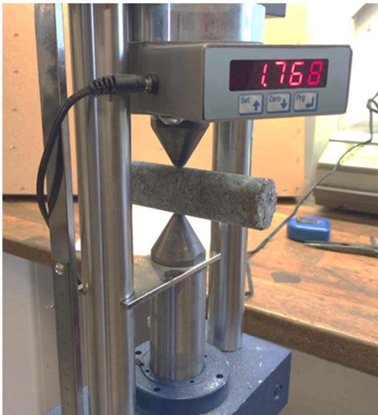
Figure 2-1. Drill core mounted for testing with Point Load Tester (PLT).
