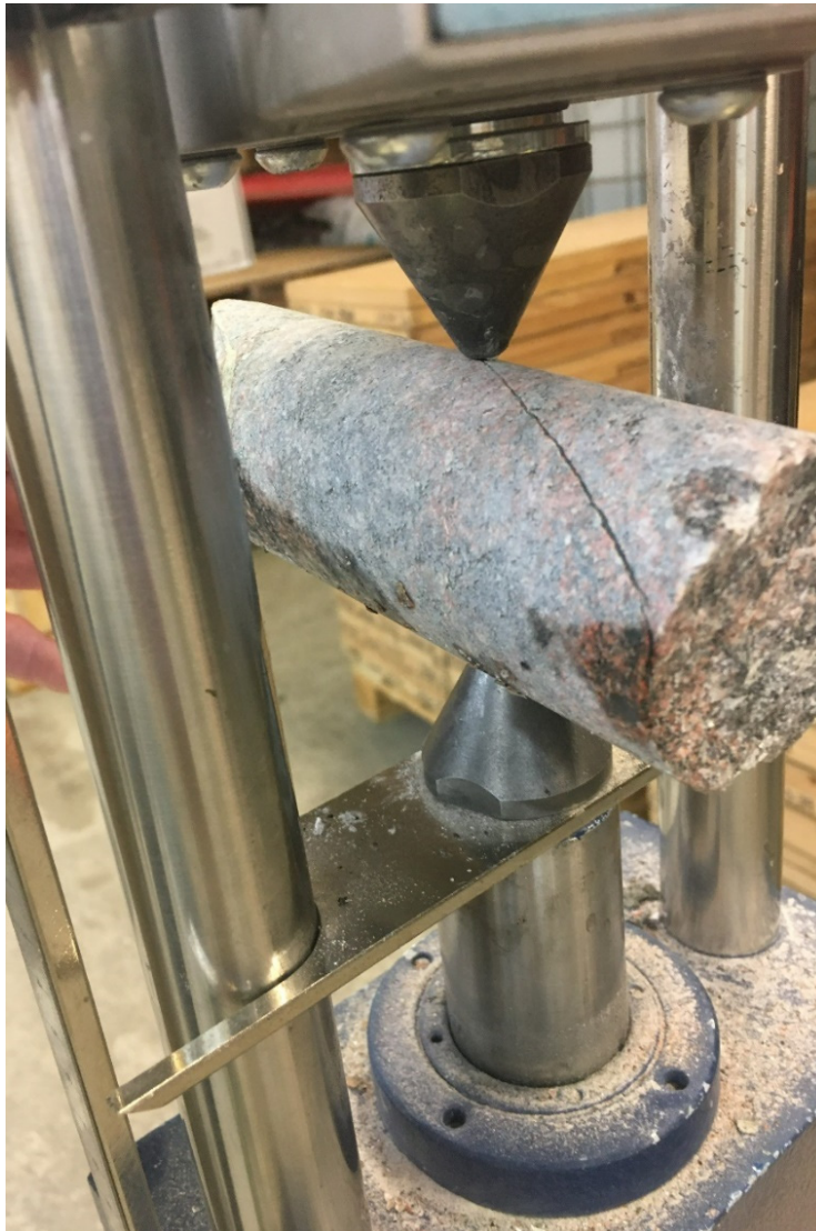
Figure 3-1. A drill core mounted in the PLT-apparatus for testing of sealed fracture strength.
