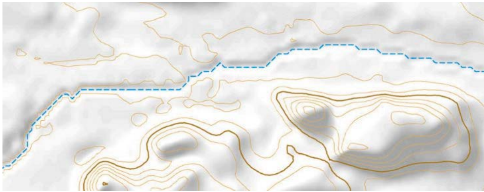
Figure 2-43. Hillshade of a terrain with eroded river channel. The channel centreline is shown as blue dashed line.
