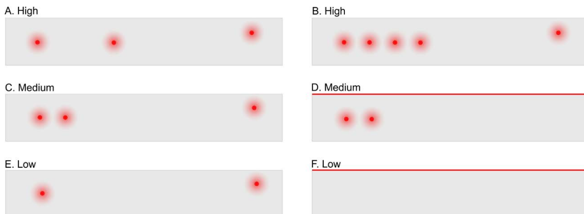
Figure 6-1. The principle of confidence assignment based on the distribution of observation points illustrated by schematic views of highly simplified deformation zones (grey rectangles). Example A shows an even distribution of observation points (red dots). Locally increased density, as in example B, does not affect the confidence level. Examples C and D show clustered observation points with one outlier, where the lineament (red line) in example D counts as an outlier. Example E shows two observation points and example F a single lineament.
