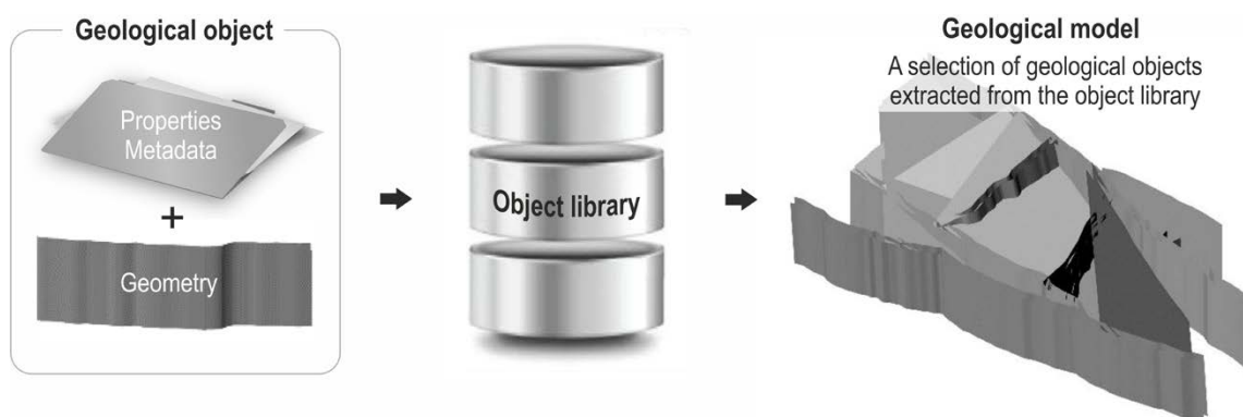
Figure 1-6. Illustration of the concept of a geological object that consists of the geometry and its corresponding metadata. The object is stored in a spatial object library from where it can be checked out, edited and re-entered with full traceability.
