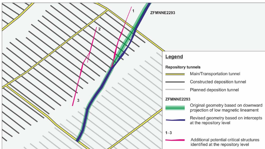
Figure 5-10. Part of the repository area showing three deterministic deformation zones. ZFMNNE2293: Originally based on downward projection of a low magnetic lineament this zone has been subjected to a geometrical adjustment based on tunnel intercepts; the name and overall geometry is still the same. 1: A splay to ZFMNNE2293, which has been modelled as a separate zone based on tunnel intercepts. 2 and 3: Two separate parts of a zone identified during the excavation of a deposition area. All zones are modelled with variable thickness.
