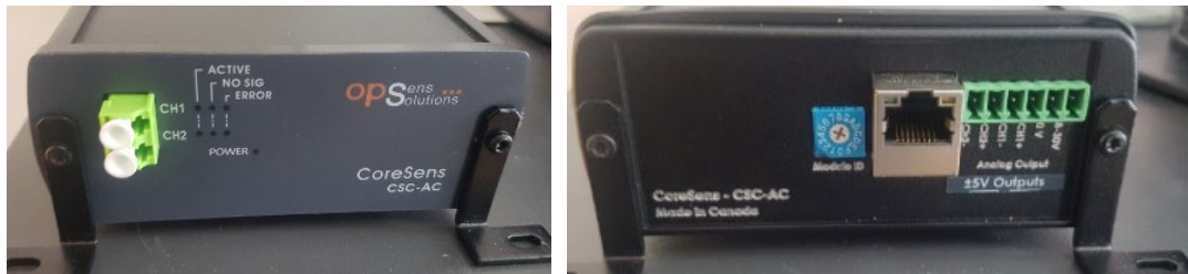
Figure 7-3. CoreSens Read-out unit front (left) and back (right). The data export can be made using Ethernet 10/100 Base T-interface or analogue output (0-5V, \pm 5V , 0-10 V, 0-20mA or 4-20mA) as seen in the right photo.
