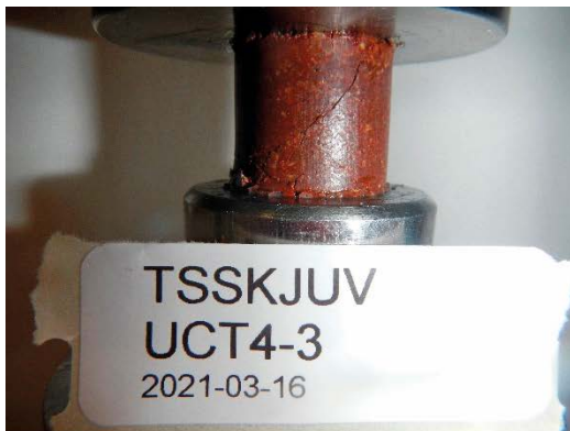
Figure A8-9b. Photos of specimens of Asha505 heated at unsaturated conditions. Test series UCT4.
