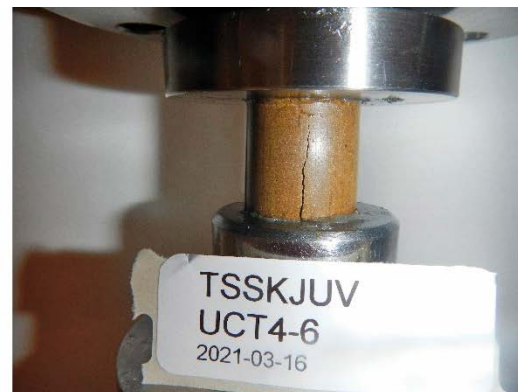
Figure A8-9c. Photos of specimens of Calcigel heated at unsaturated conditions. Test series UCT4.
