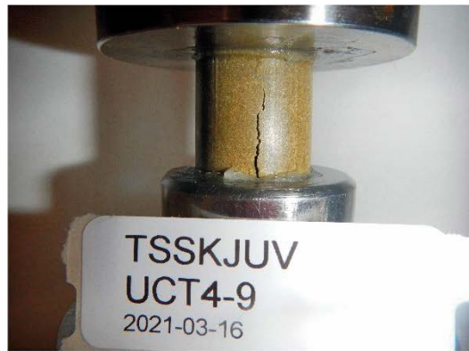
Figure A8-9e. Photos of reference specimens of Asha505 (left) and Calcigel (right). Test series UCT4.
