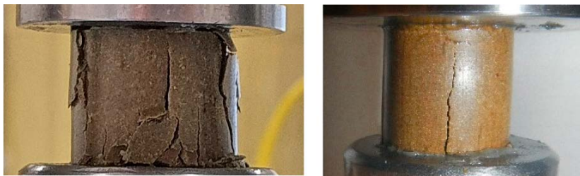
Figure 4-61. Specimens of Calcigel. To the left heated at saturated conditions (UCT3-2) and to the right specimen from the reference series (UCT4-6).
