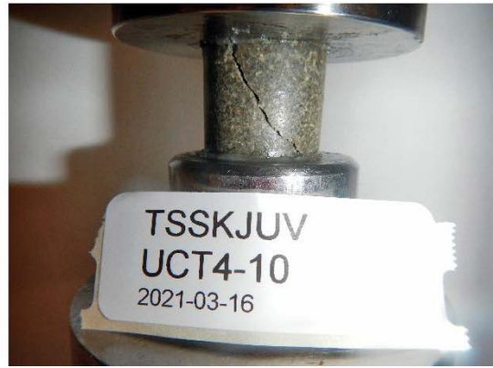
Figure A8-9d. Photos of reference specimens of MX-80. Test series UCT4.
