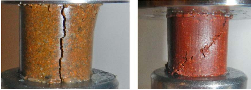
Figure 4-60. Specimens of Asha505. To the left heated at saturated conditions (UCT2-2) and to the right from the reference series (UCT4-4).
