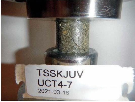
Figure A8-9d. Photos of reference specimens of MX-80. Test series UCT4.
