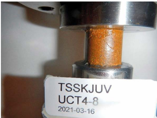
Figure A8-9e. Photos of reference specimens of Asha505 (left) and Calcigel (right). Test series UCT4.
