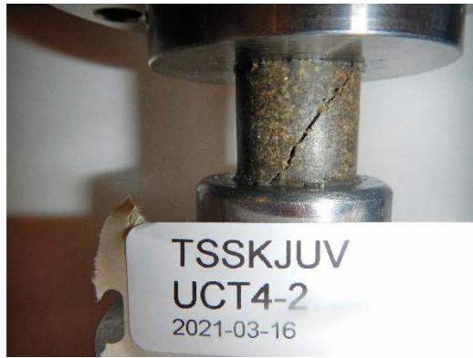
Figure A8-9a. Photos of specimens of MX-80 heated at unsaturated conditions. Test series UCT4.
