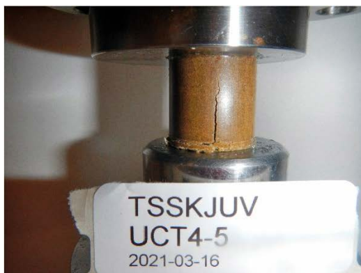
Figure A8-9c. Photos of specimens of Calcigel heated at unsaturated conditions. Test series UCT4.
