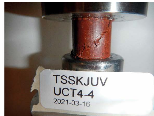
Figure A8-9b. Photos of specimens of Asha505 heated at unsaturated conditions. Test series UCT4.
