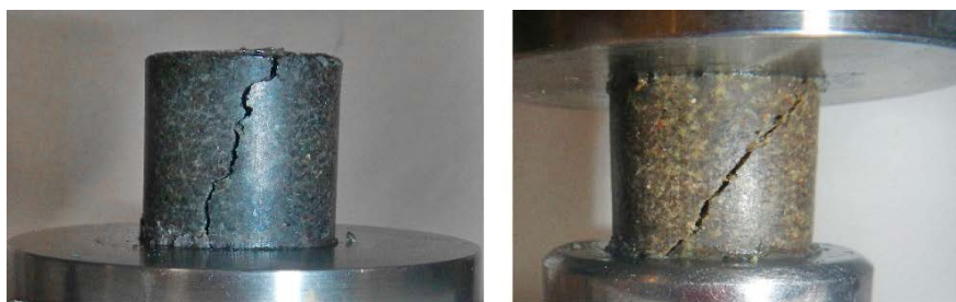
Figure 4-59. Specimens of MX-80. To the left heated at saturated conditions (UCT1-2) and to the right from the reference series (UCT4-2).
