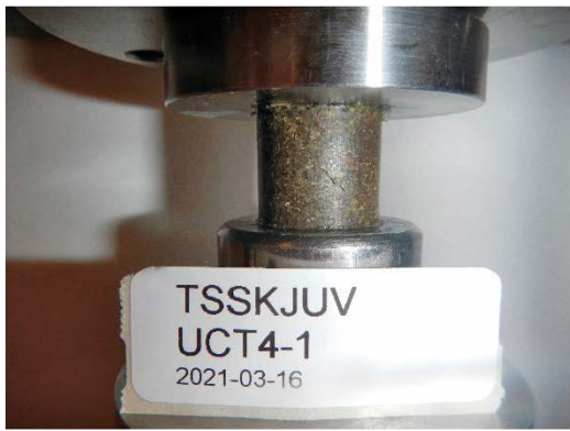
Figure A8-9a. Photos of specimens of MX-80 heated at unsaturated conditions. Test series UCT4.
