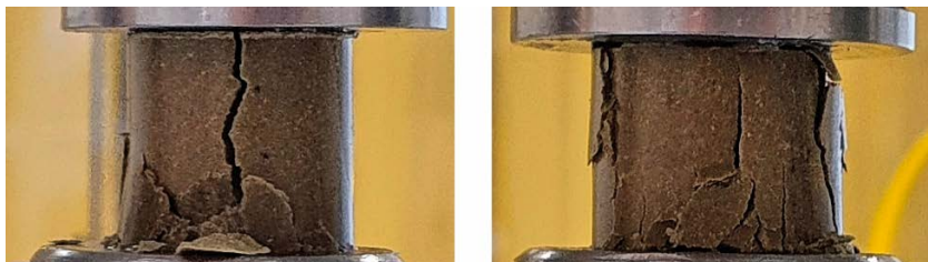
Figure A8-8. Photos of specimens of Calcigel heated at saturated conditions, test series UCT3.
