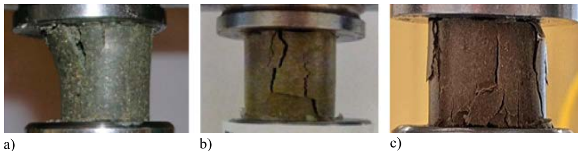
Figure 5-19. Examples of failure without continuous surfaces going through the specimen, but rather with local fractures: a. MX-80 (specimen F124 exposed to 20^\circ\text{C} , Dueck 2010), b. Calcigel, (TMS A2 exposed to 20^\circ\text{C} , this study), c. Calcigel (UCT3-2 exposed to 240^\circ\text{C} , this study).
