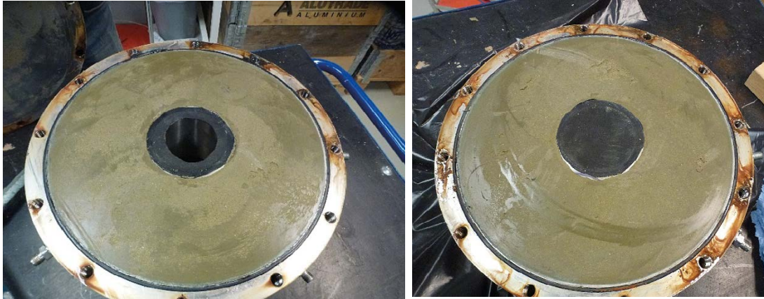
Figure A2-3. The bentonite cylinder ring at dismantling with the upper side (left) and the lower side (right) with the rubber sealings left. The centre cylinder is located in the centre of the device, the photos are somewhat misleading.
