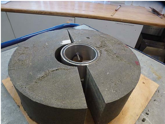
Figure A2-15. The block was divided in two parts before the sampling for determination of water content and bulk density.
