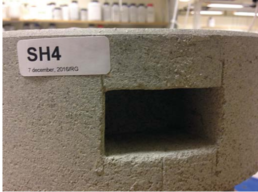
Figure A2-11. Cavity in the block used for test SH4. A second cavity was cut out on the other side of the block.
