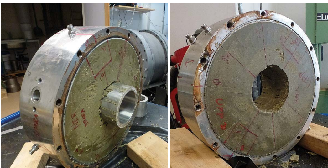
Figure A2-5. The inner steel cylinder is almost (left) and completely (right) removed.
