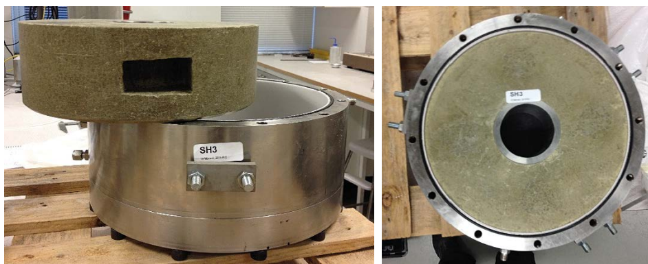
Figure 5-1. Photos of the bentonite block used for SH3. The bentonite block with the cavity (left) and installed into the test device (right).
