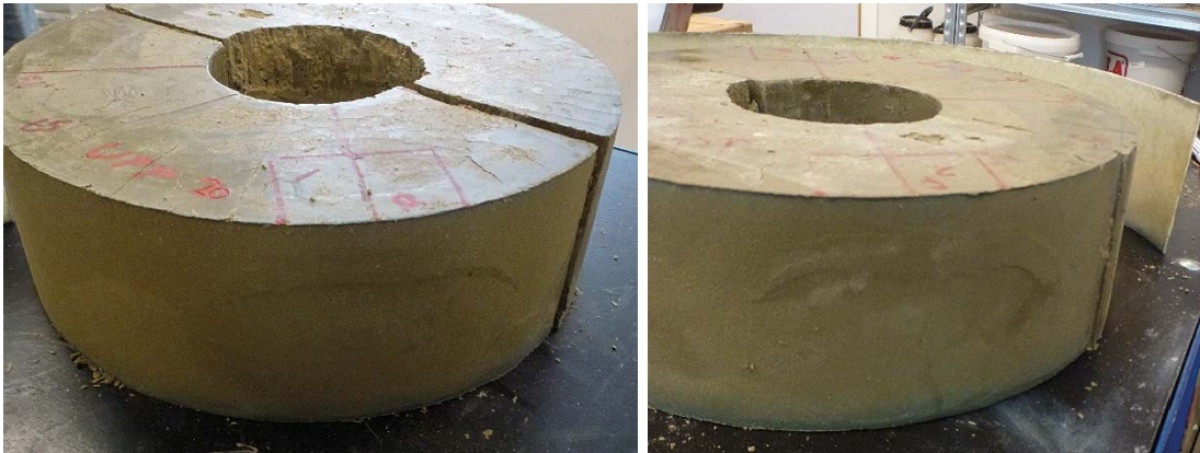
Figure A2-7. Photos of each of the two cavities after removal of the radial filter.
