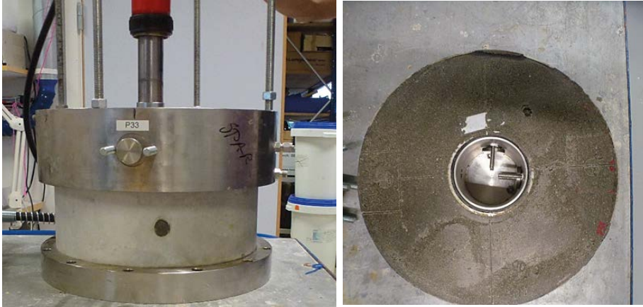
Figure A2-14. A hydraulic jack was used for the dismantling of the block (to the left) and the dismantled block with the inner steel cylinder left (to the right).
