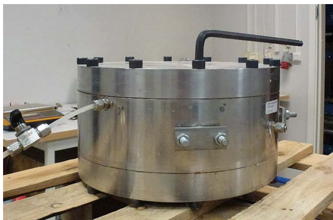
Figure A2-2. The confined cylinder at dismantling.
