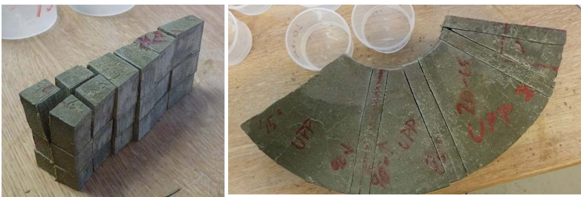
Figure A2-8. Sampling was made within a sector and along lines. The sector was divided into four wedges A to D and one of these is shown (left). Sampling was made at the angles 0, 20, 65 and 90 degrees from the centre of the cavity and the lines L0, L20, L65 and L90 are marked (right).
