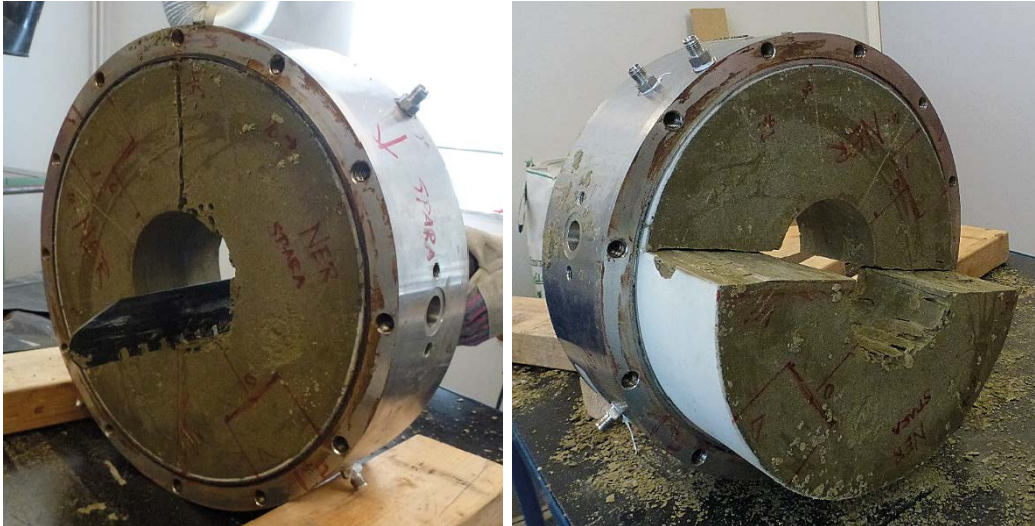
Figure A2-6. The bentonite cylinder is sawn (left) into two half cylinders (right).
