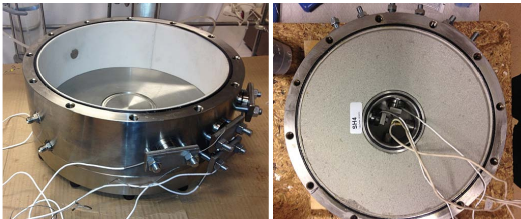
Figure A2-12. The device with filter and sensors used for the test (to the left) with the installed block (to the right).
